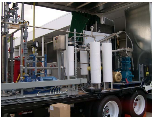
Figure 9: Picture of compressor (K101) and the coalescers / catch tanks.
