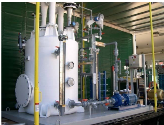
Figure 6. Picture of flue gas scrubber (C301).
