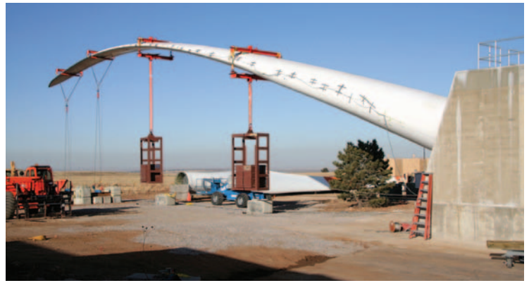
A 44.5-meter blade static test performed at the NWTC. PIX14708
