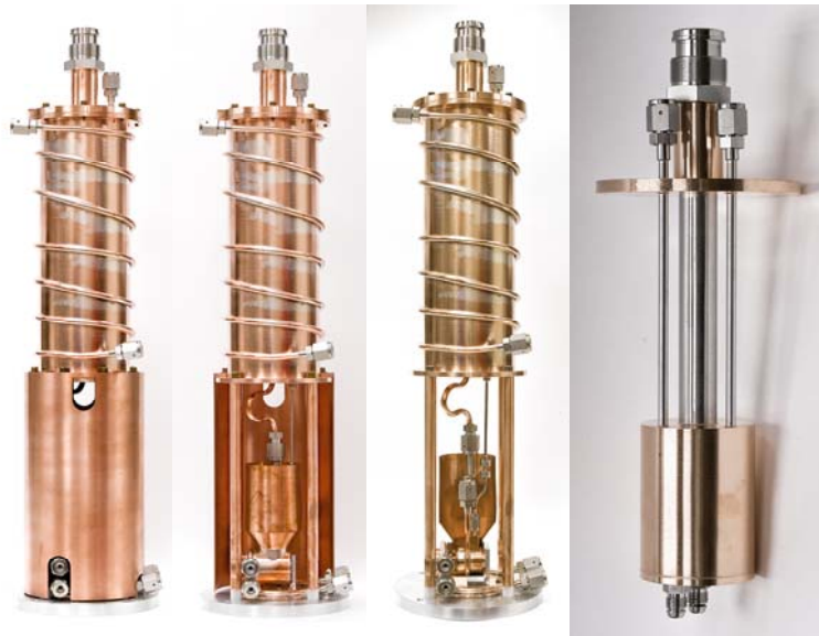
Figure 12. Left: Basic test cell system with radiation shields in place and removed; Right: Cryostat removed from upper radiation shield.
