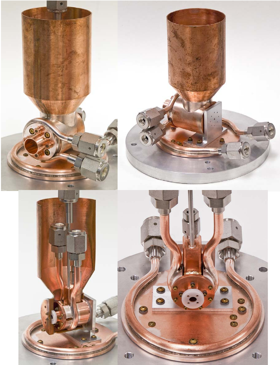
Figure 13. Views of basic test cell assembly on mounting plate.
