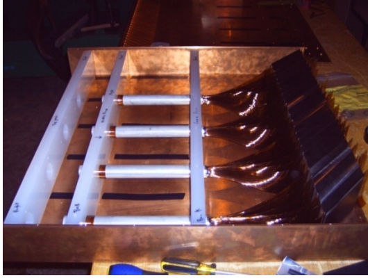
Fig. 6. The lightguides, quartz fiber bundles, and tungsten plates in the interior of a ZDC Hadronic module during assembly at CERN.
