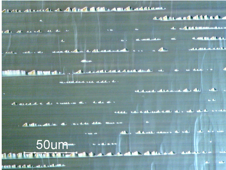
Fig. 5. Nomarski optical micrograph of a nearly coalesced a -plane LEO sample.
