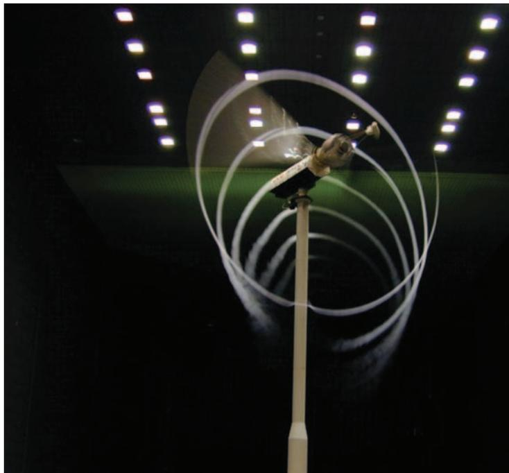
Wind turbine smoke test in the NASA Ames 80 ft x 120 ft wind tunnel.
