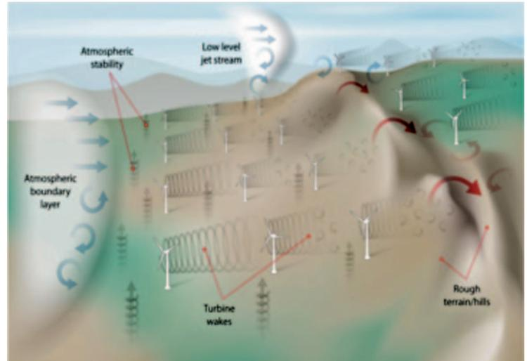
Schematic of wind farm interactions with atmospheric boundary layer, terrain, and vegetation.
