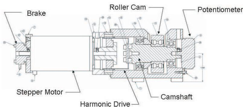
Figure 1: Cross section of roller cam module
