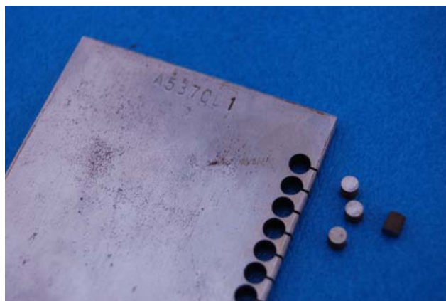
Figure 1. Starting ASTM A537 Class 1 carbon steel coupon and electrodischarge-machined specimens.
