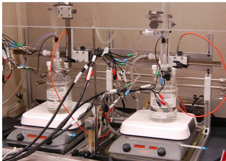
Figure 4. Experimental apparatus for open-circuit potential measurements.
