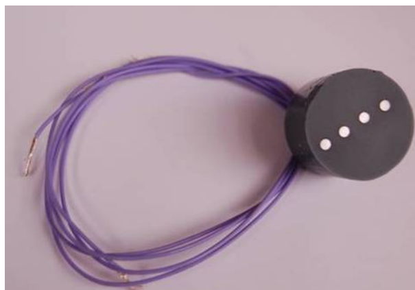
Figure 2. Array of four specimens mounted in metallurgical mounting compound.
