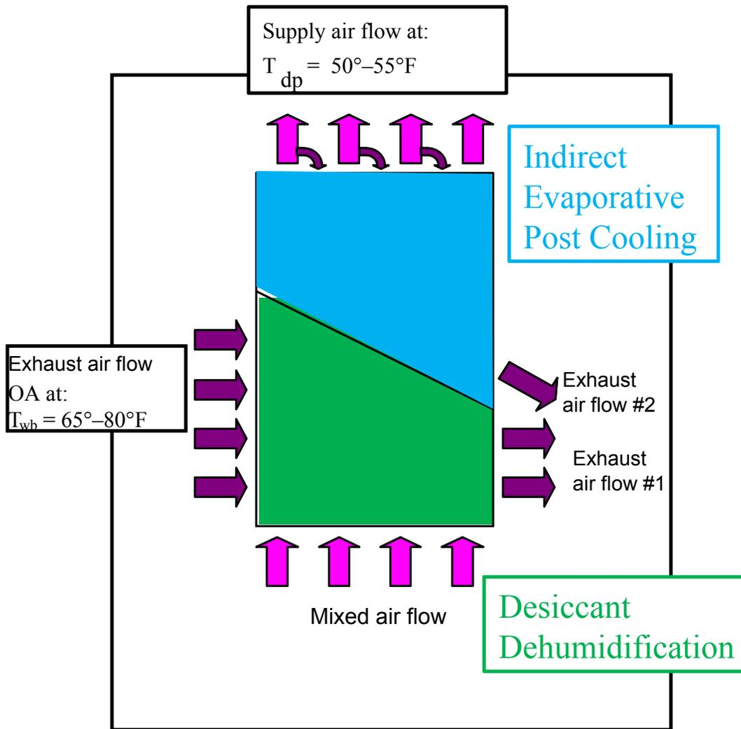
**Figure 2-11 DEVap HMX air flows**
