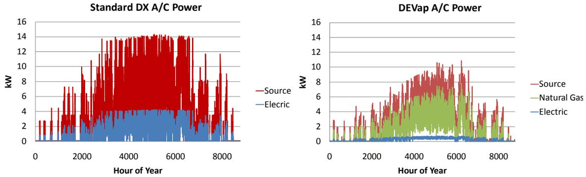
**Figure 3-13 A/C power comparison in Houston for residential new construction**
