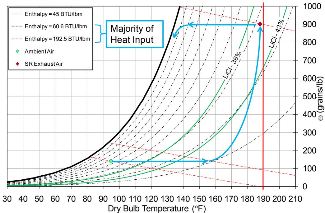
**Figure 2-5 Desiccant reactivation using single-effect scavenging air regenerator**
