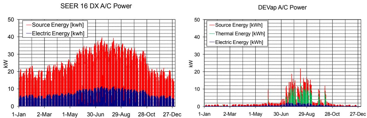
**Figure 3-21 A/C power comparison for a small office benchmark in Phoenix**
