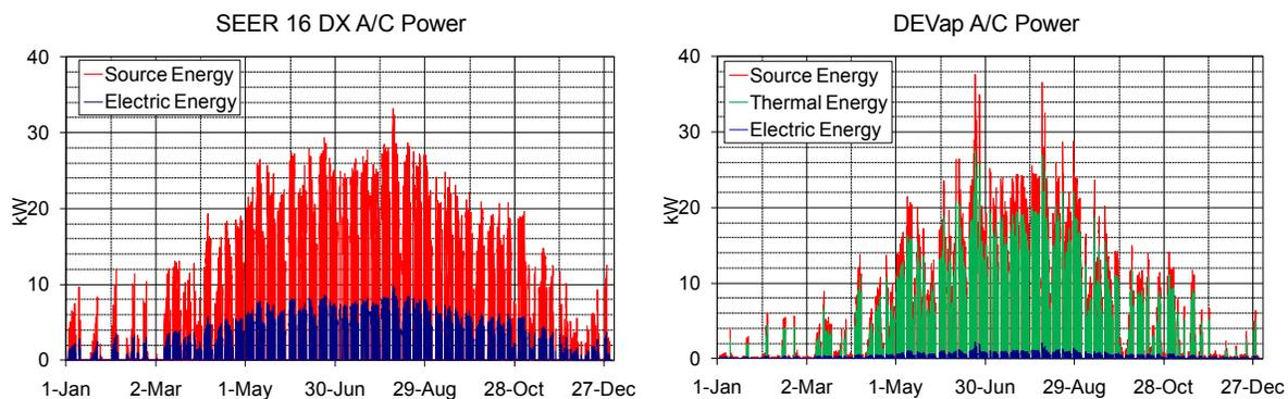
**Figure 3-22 A/C power comparison for a small office benchmark in Houston**
