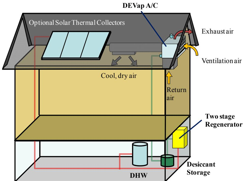
**Figure 2-14 Example diagram of a residential installation of DEVap A/C showing the solar option (green lines represent desiccant flows)**
