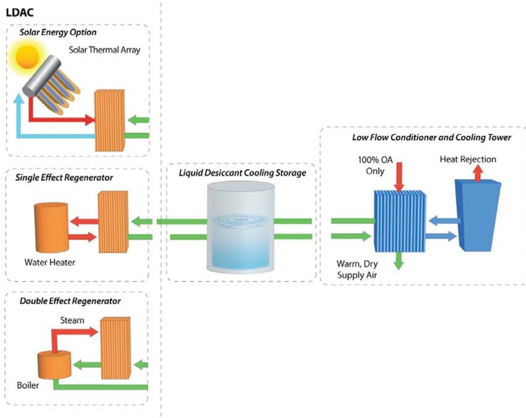
**Figure 2-7 LDAC schematic**
