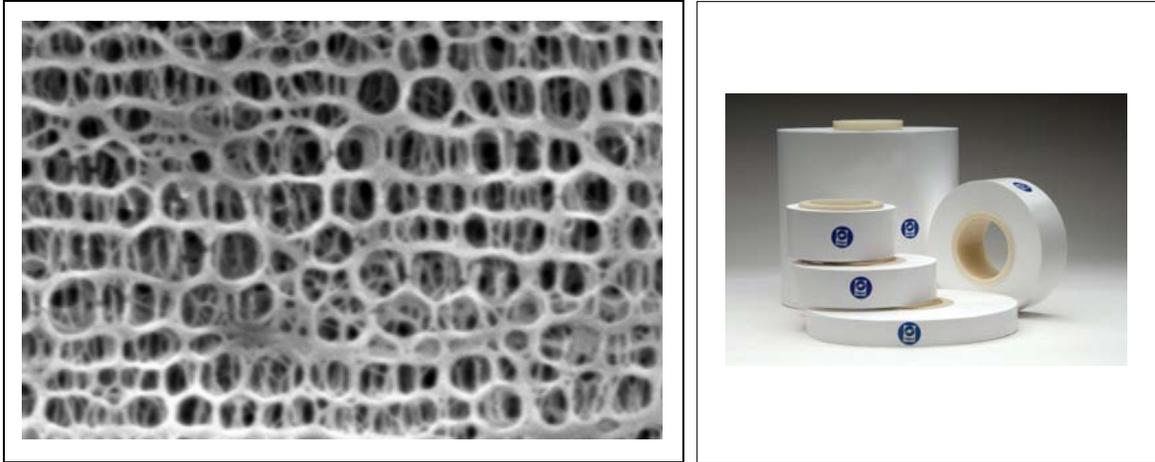
**Figure 2-10 Scanning electron microscope photograph of a micro porous membrane (Patent Pending, Celgard product literature)**
