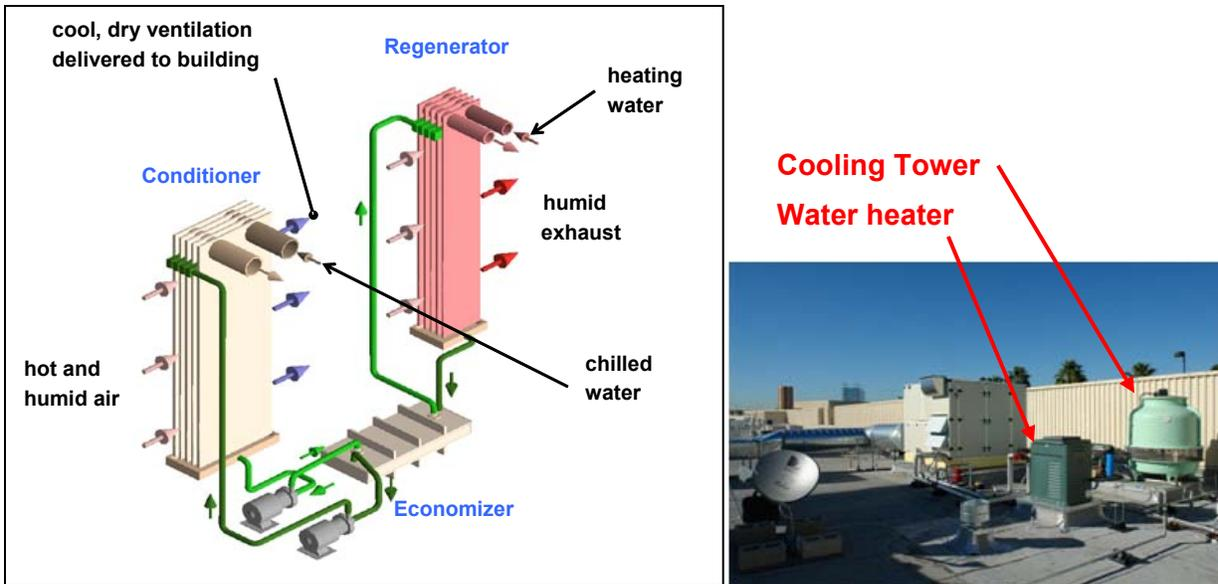
**Figure 2-6 Major components and packaging of the AILR LDAC (Photograph shows packaged HMXs, water heater and cooling tower)**
