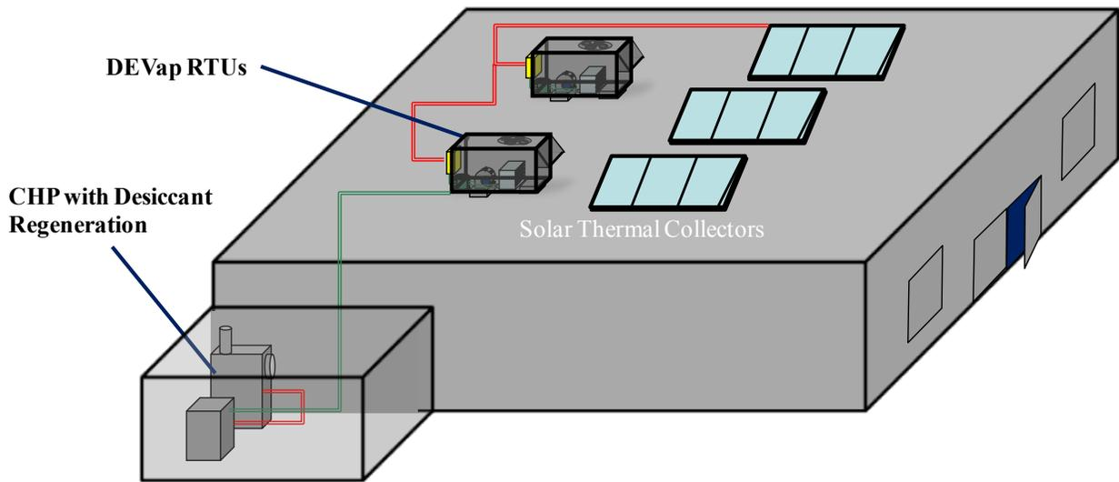
**Figure 2-16 Example diagram of a commercial installation of DEvap A/C showing the solar and CHP options**
