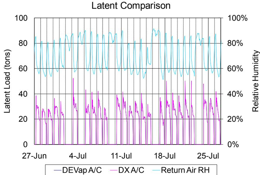
**Figure 3-12 Latent load comparison and resultant space RH in Houston**
