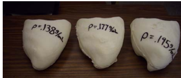
Fig. 24. A few polyurethane foam models which were cast using the lung mold. The highest density foam lung created so far is 0.195 \text{ g/cm}^3 .
