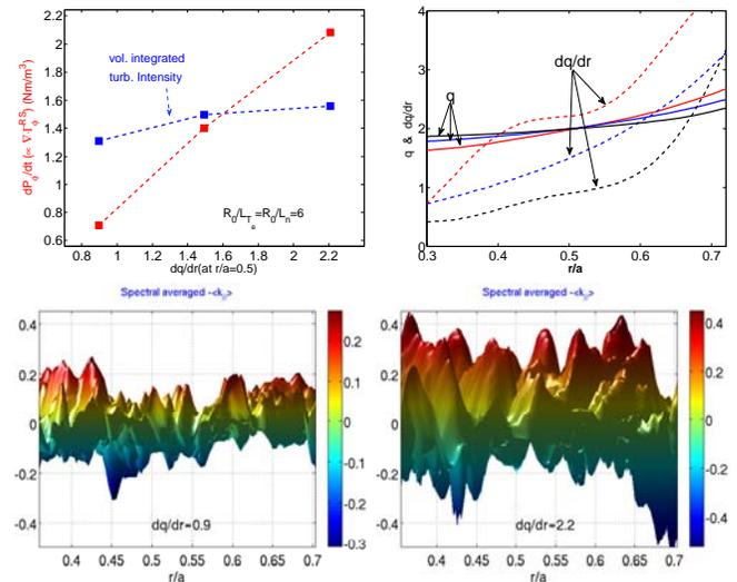
FIG. 3: CTEM-driven total intrinsic torque versus the radial variation of  $q$  averaged over the central core region (upper-left), corresponding radial profiles of  $q$  and  $dq/dr$  of the three equilibria used for these simulations (upper-right), and spatio-temporal images of spectrum-averaged  $\langle k_{\parallel} \rangle$  for two cases with averaged  $dq/dr = 0.9$  (lower-left) and  $dq/dr = 2.2$  (lower-right) – these are 2D views in the  $\langle k_{\parallel} \rangle$ - $r$  domain.
