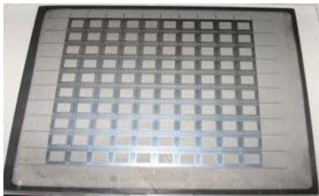
**Figure 1. Array of CdTe PV cells on 6"x6" substrate**
