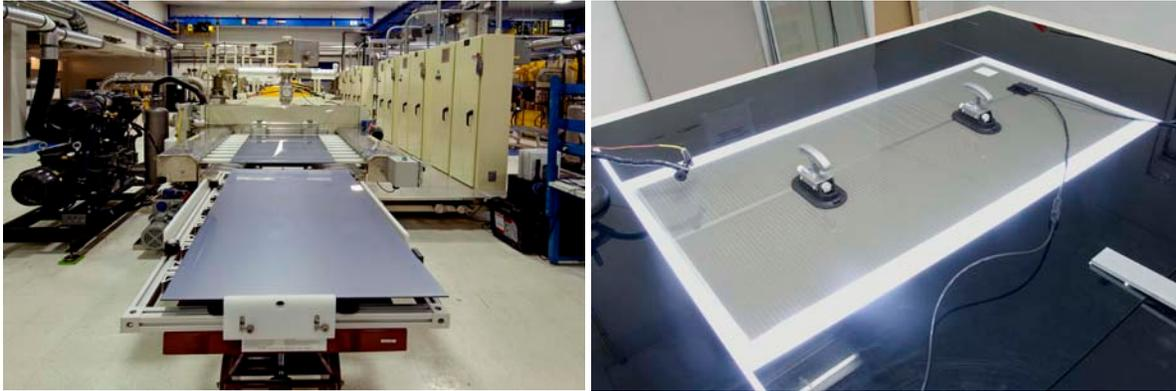
**Figure 5. CdTe process equipment exit and a completed module in J-V testing.**
