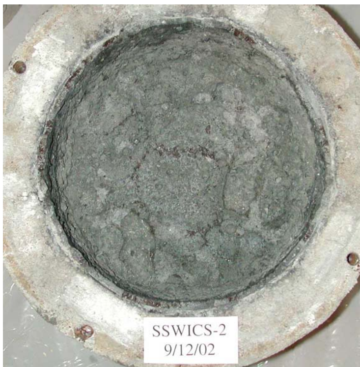
Figure 7.1 Solidified corium within MgO liner (top view).
