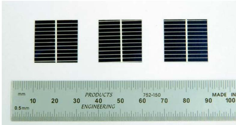
Figure 7. Three solar cells fabricated on Direct Wafers, 4 cm<sup>2</sup> each. Credit: 1366 Technologies.
