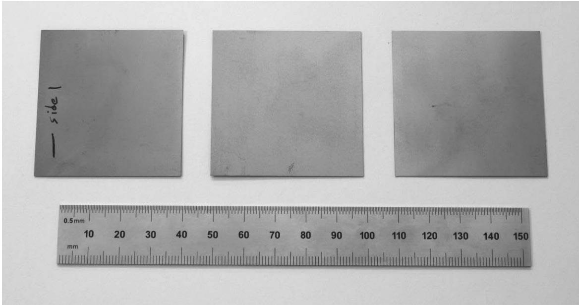
**Figure 6. Silicon Direct Wafers submitted to NREL for Deliverable 2 with flat, smooth surfaces, average thickness  $\sim 200\ \mu\text{m}$  with deviation  $< 20\%$ . Credit: 1366 Technologies.**
