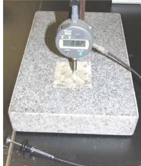
**Figure 2: Thickness measurement.**
