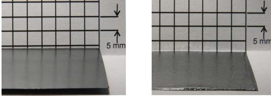
Figure 3. Surface quality on two sides of a silicon Direct Wafer. Credit: 1366 Technologies.
