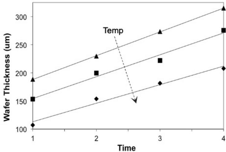
Figure 5. Measured thicknesses of silicon wafers as a function of process parameters of temperature and time.
