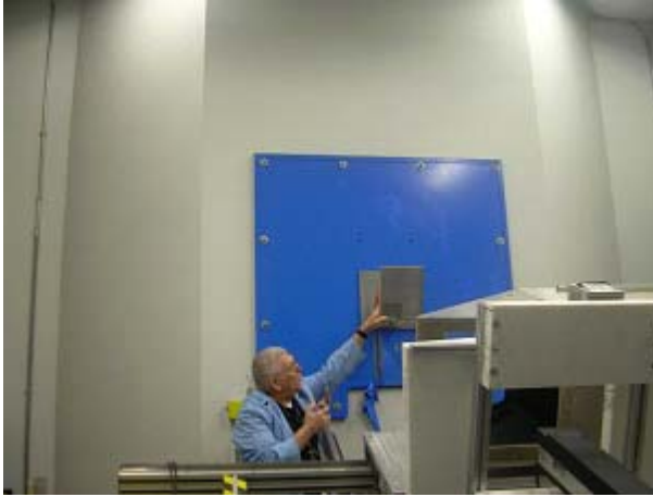
Fig. 19 (a) Photo of the placement of the Fuji Film Imaging detector at the beam stop and alignment laser position, which is the maximum 5.3 meter distance downstream of the PMF entrance (with second collimation slit).
