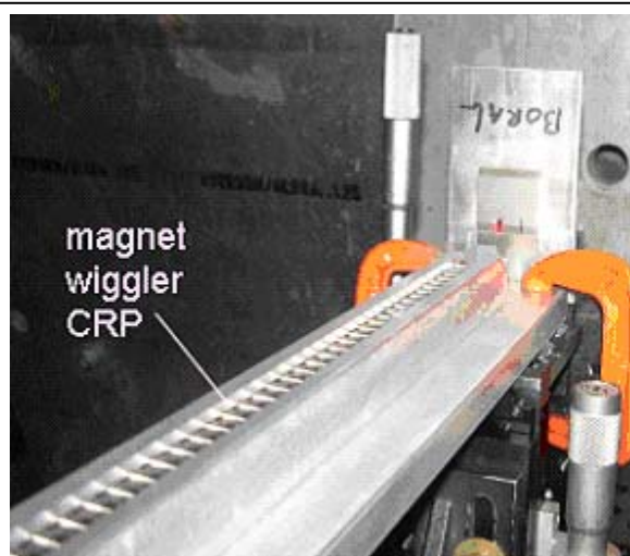
Fig. 4. Picture of the magnetic wiggler CRL in place at the MNRC beam line. The neutron beam enters from the circular aperture at the right, passes through the Gd slits and then over the top of the prism. The individual periods of the compound prism form the ladder-like appearance of the device.
