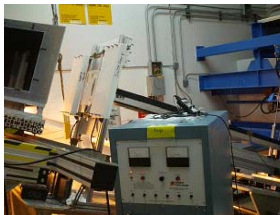
Fig 18 (c) Shown is a photo showing the placement of the Fuji imaging plate at the end of the PMF between the two rectangular borated polyethylene limiting apertures.
