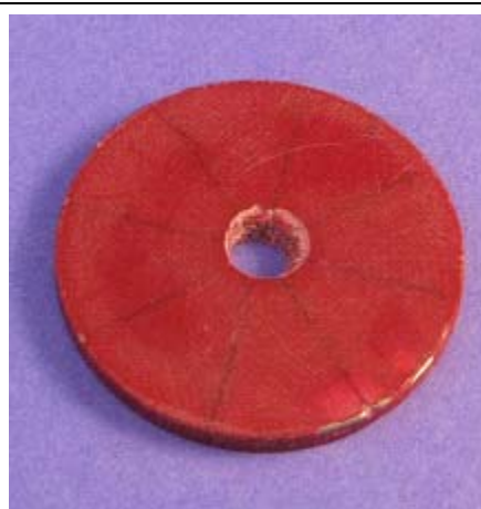
Fig. 11 Shown is a photo of a two dimensional PMF with alternating N-S-N-S radial magnetic field.
