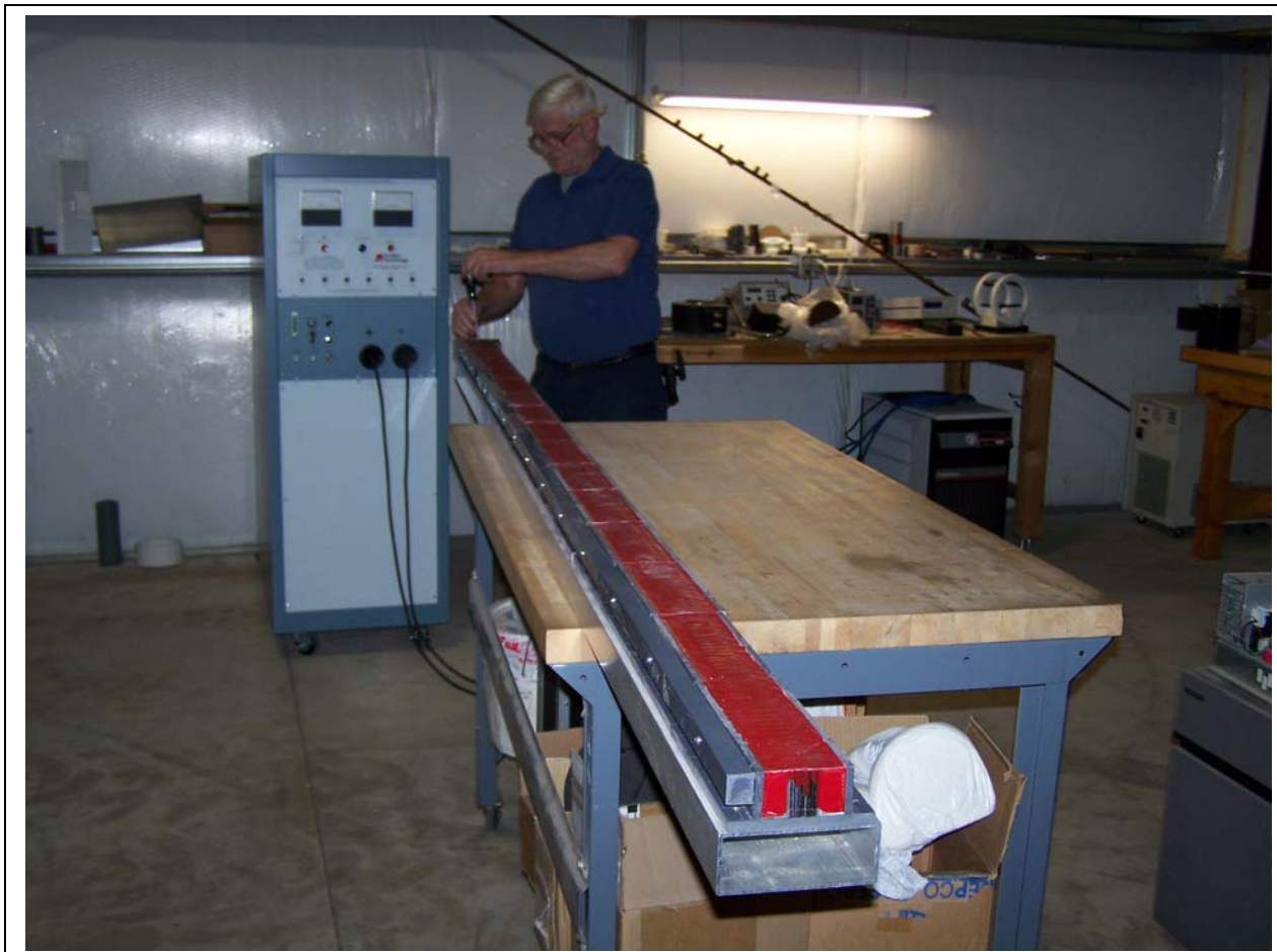
Fig. A5 Photo of electromagnetic PMF being tested at the Oersted facility in Troutdale, Oregon.
