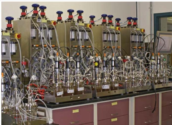
The 500-mL Biostat Q-Plus fermentors are used for small-scale fermentation testing. Photo by Cindy Gerik, NREL/PIX 19431
