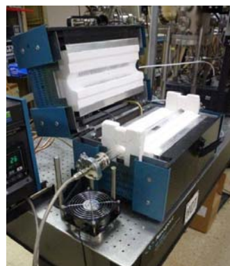
Figure 1. SWNT growth furnace
