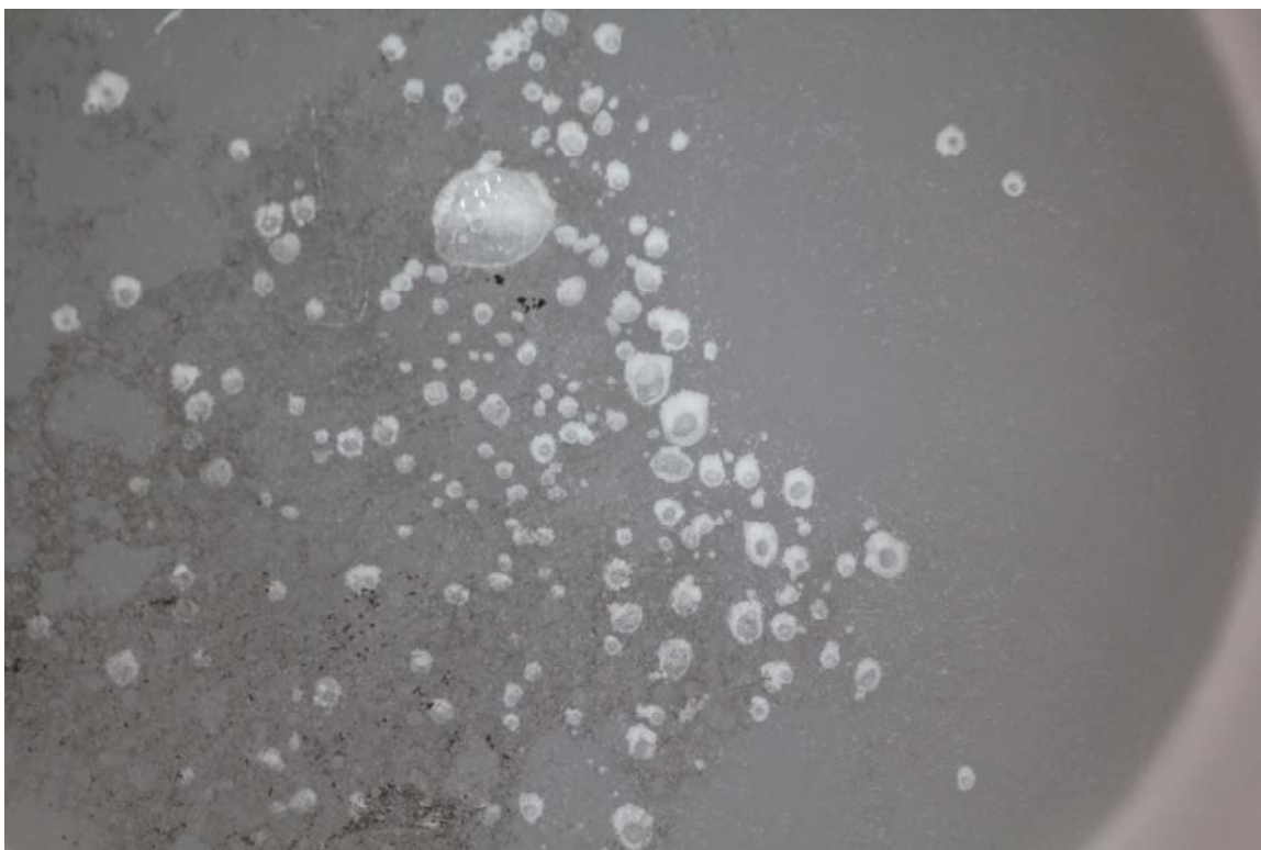
Figure 22. CO 2 -in-water emulsion at high slurry concentration with other conditions as described above. CaCO 3 particles are visible as a thick layer around individual droplets.
