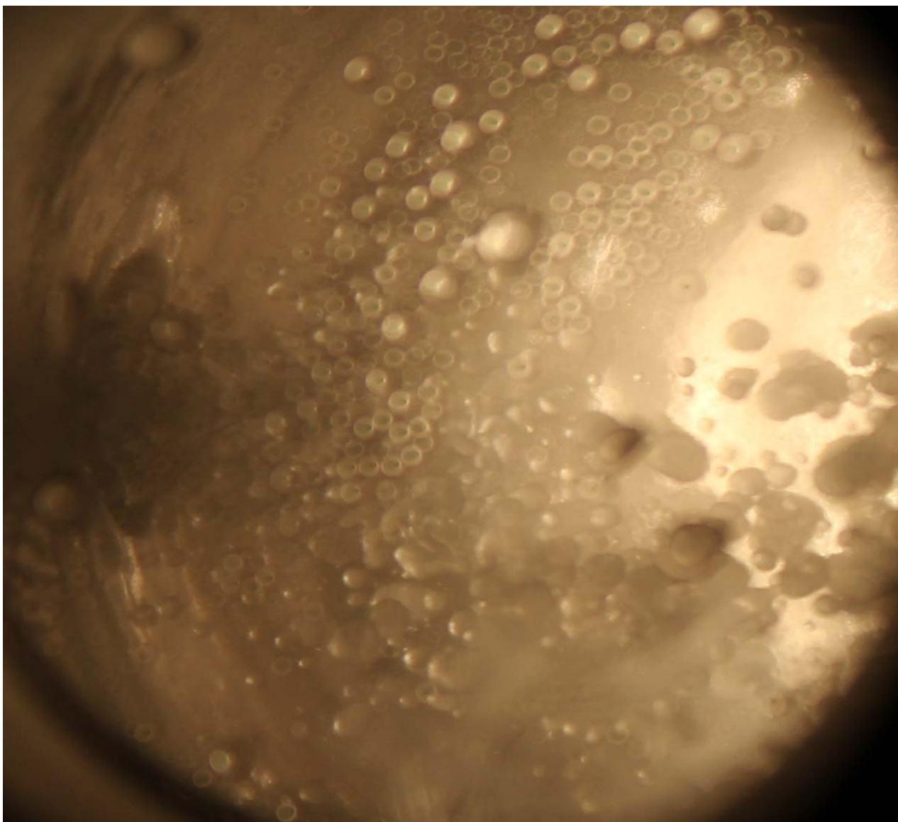
Figure 5. Water-in-Supercritical CO 2 Emulsion Stabilized by Teflon Particles. Globule size 200 – 300 \mu\text{m} .
