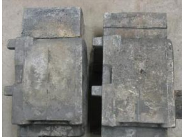
Figure 10.1 View on top surface of casting produced in industrial confirmation trials.
