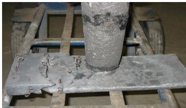
Figure 6.3 Incomplete filled casting.
