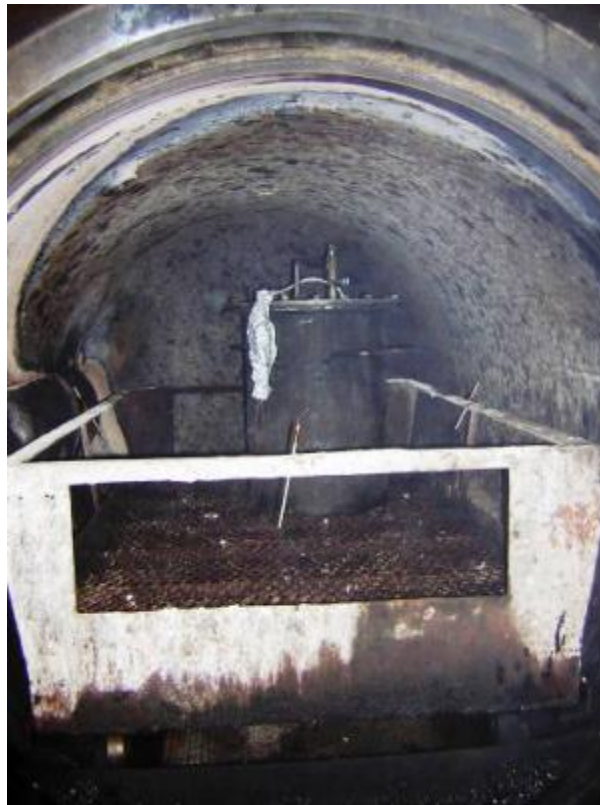
Figure 13.3 Thermocouples placed on the basket and the data logger assembly in the autoclave before the cycle.
