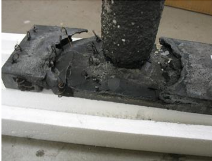
Figure 7.3 An incomplete fill. Notice the fully formed edges indicating that the metal reached the edge and then started to flow back resulting in foam engulfment
