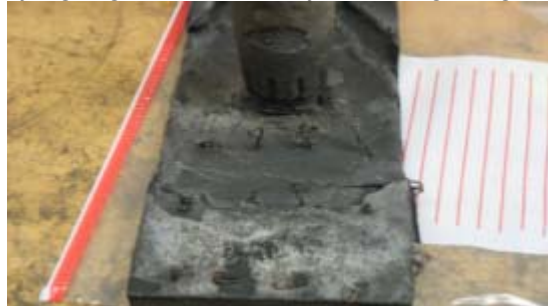
Figure 6.2 The incomplete fill with a restrictive riser neck shows that the liquid steel reaches the end wall though the bottom of the pattern and washes back over the remaining pattern.
