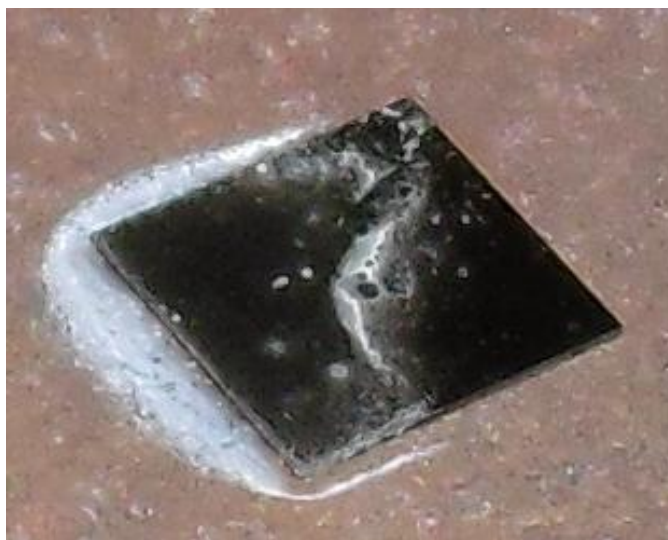
Figure 5. The SiC surface oxidation as a result of open air PTP processing.
