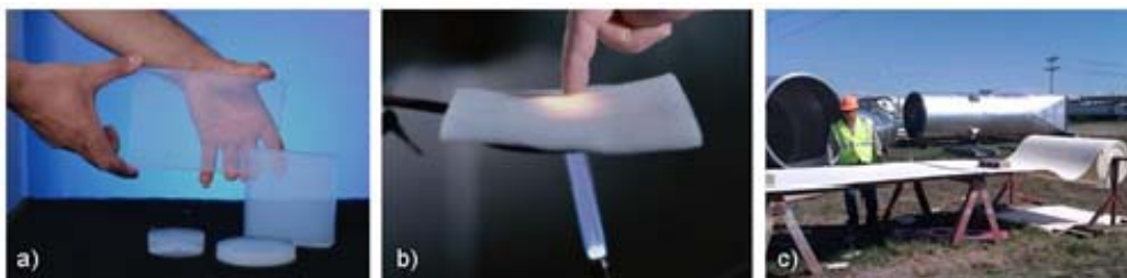
Figure 3: Aerogel: a) monolithic form, b) flexible blanket form, and c) on construction site.
