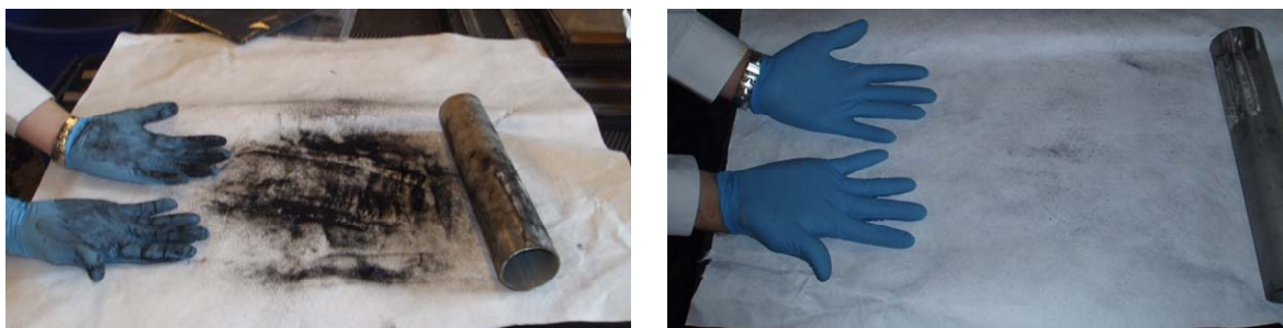
Figure 5: Dust evolution after handling Spaceloft 6250 uncoated (left) and coated (right).
