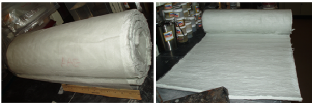
Figure 16. Pilot-line scale production of the Pyrogel HT insulation.
