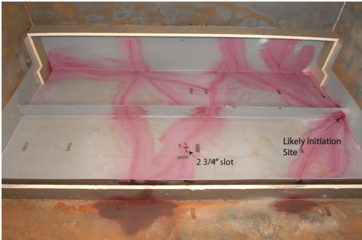
Figure 49. Interior crack formation during Test 16
