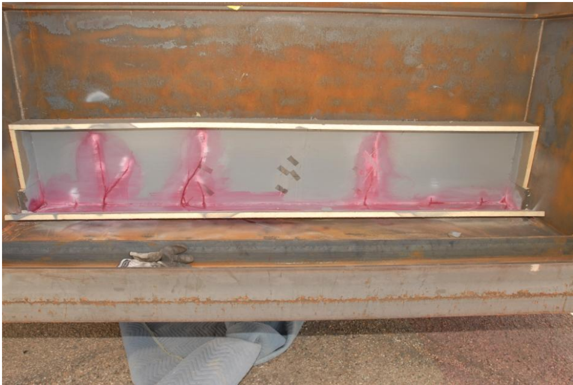
Figure 54. Outside through-cracks for Test 16
