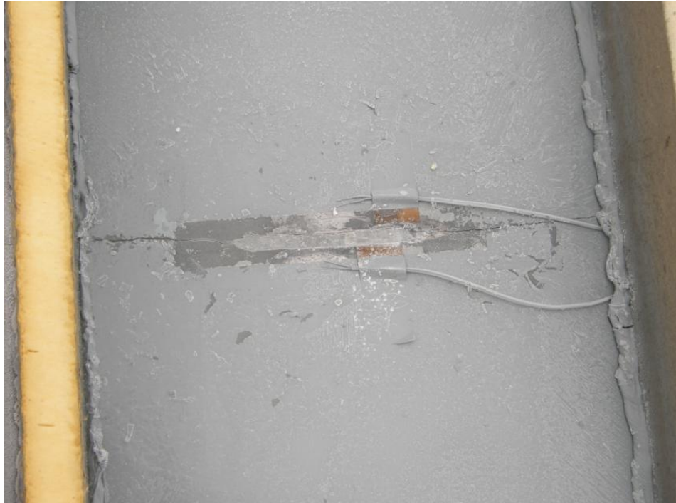
Figure 24. Cracked formed in 72 in. x 72 in. plate during Test 10
