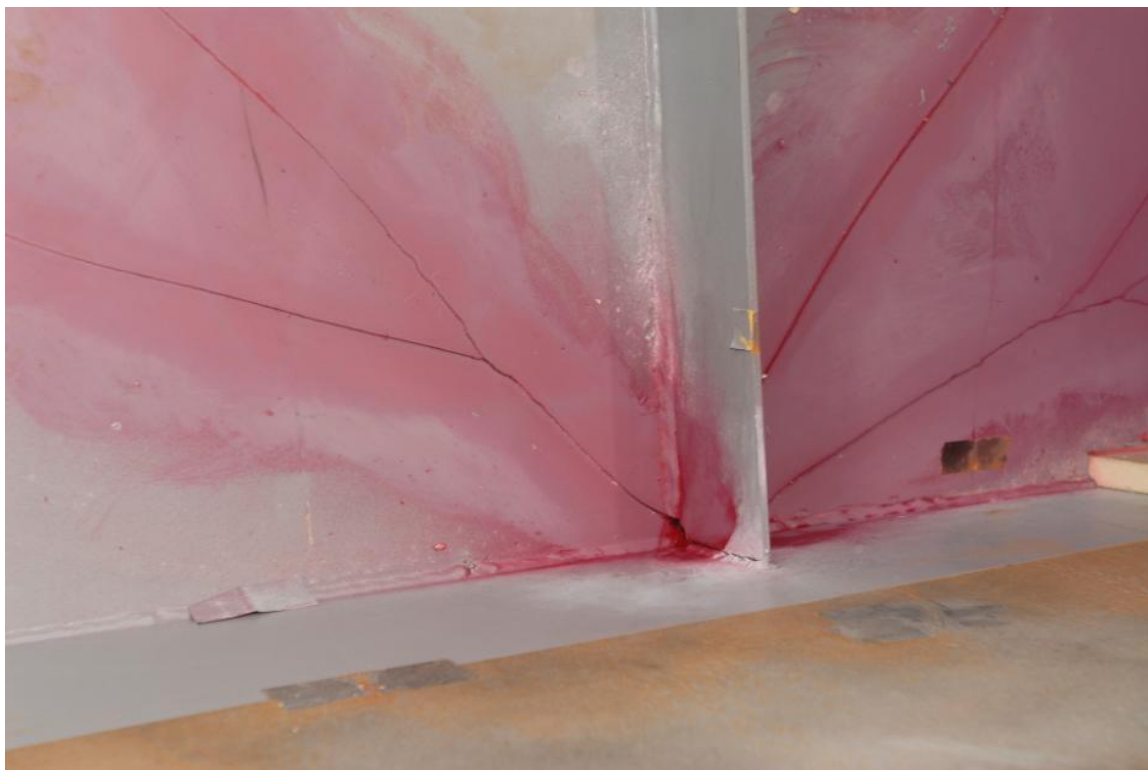
Figure 51. Close-up of likely initiation site for Test 16
