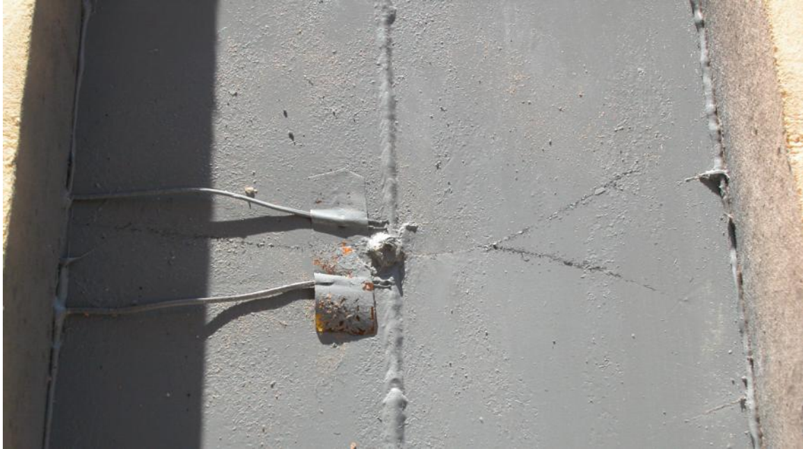
Figure 19. Crack generated in Test 6, 48 in. x 48in. x ¼ in. welded plate with notched holes
