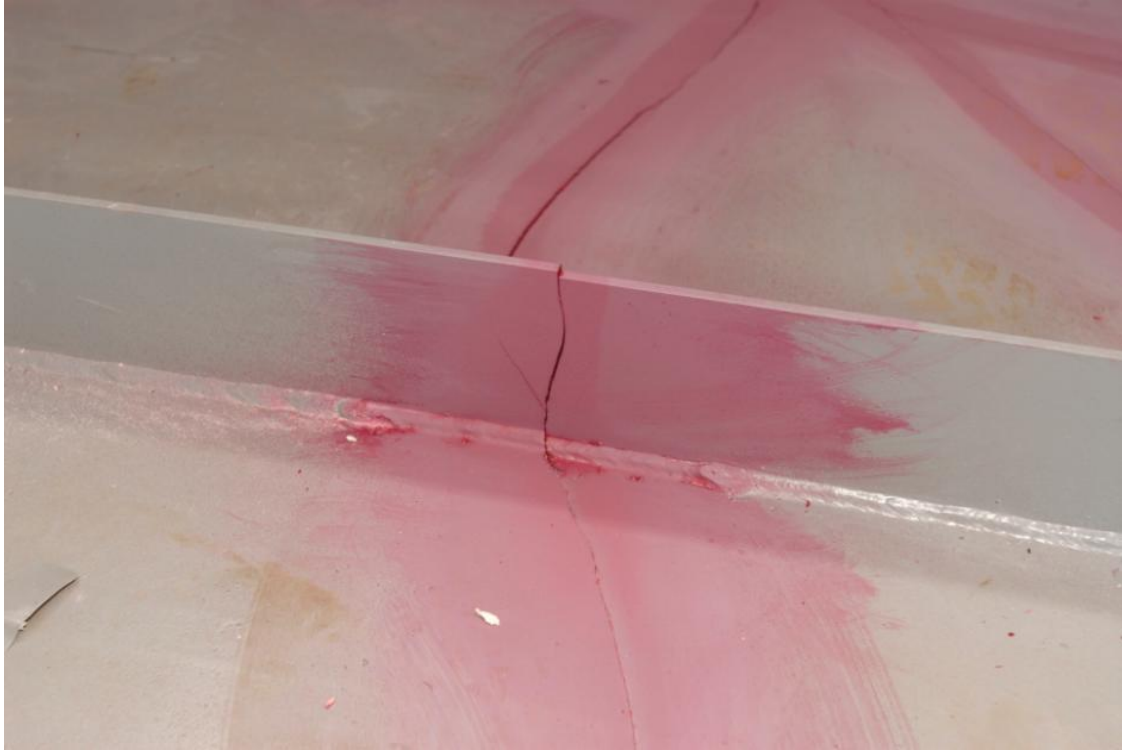
Figure 53. Close-up stiffening rib fracture for Test 16
