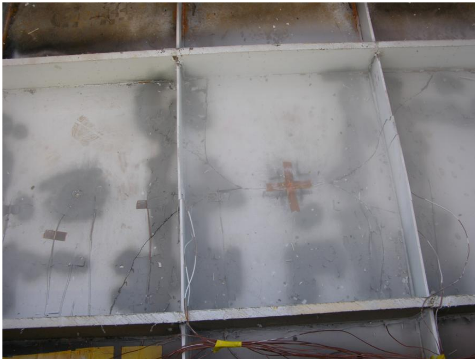
Figure 44. Crack formation during Test 14
