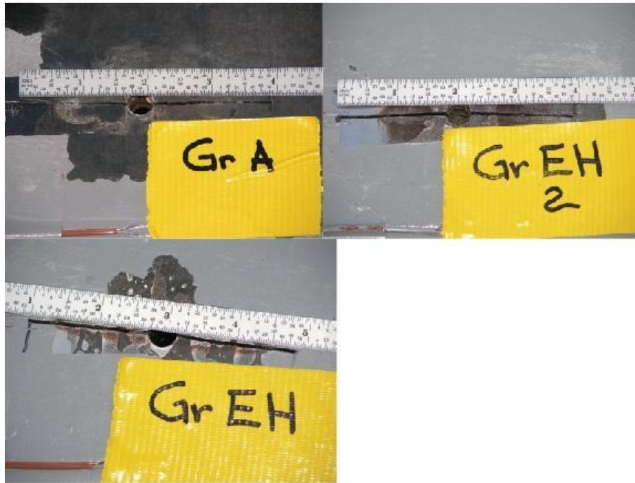
Figure 31. Notch geometry used for ABS Grade steel Phase II tests
