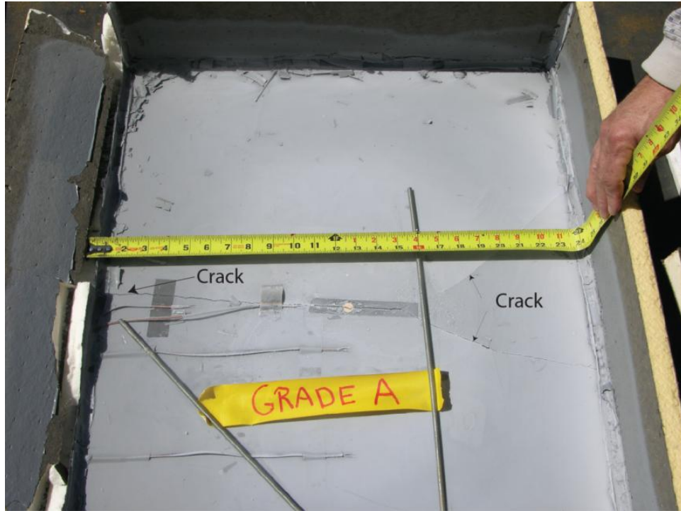
Figure 32. Cracking pattern for Test 19
