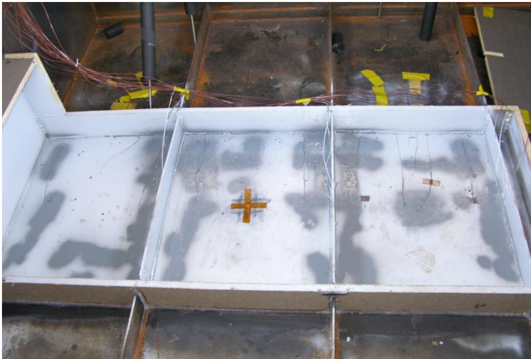
Figure 42. Trough with added notches and paint repair prior to Test 14
