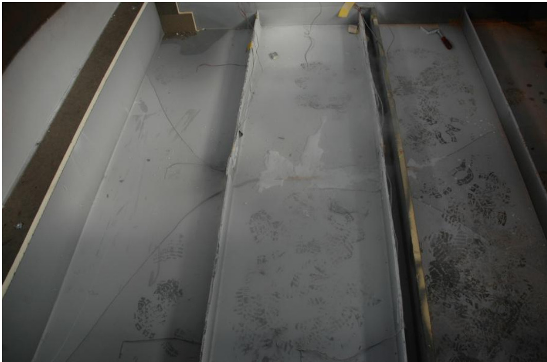
Figure 60. Crack progression for Test 23
