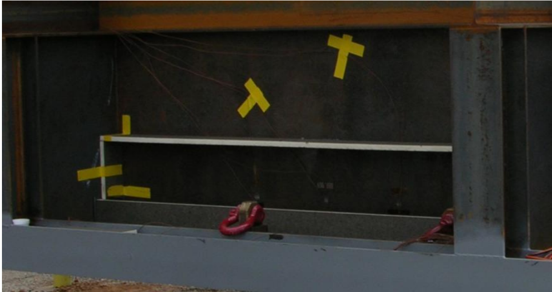
Figure 48. Trough layout outside vertical Gr. EH plate for Test 16
