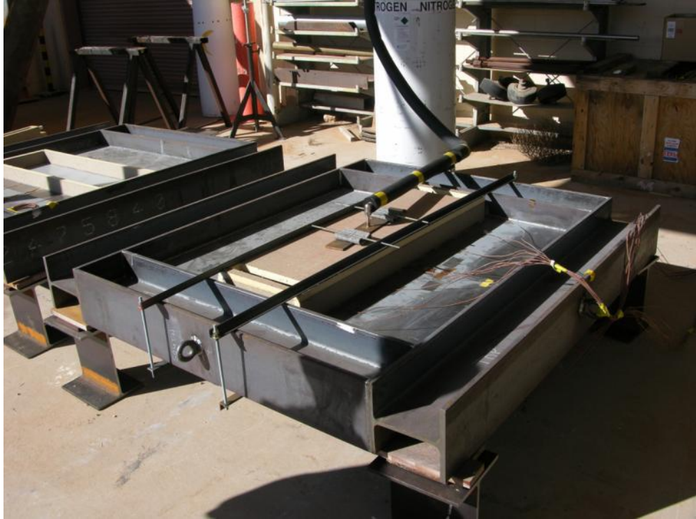
Figure 12. Test configuration for the 48 in. x 48 in. Phase II plates
