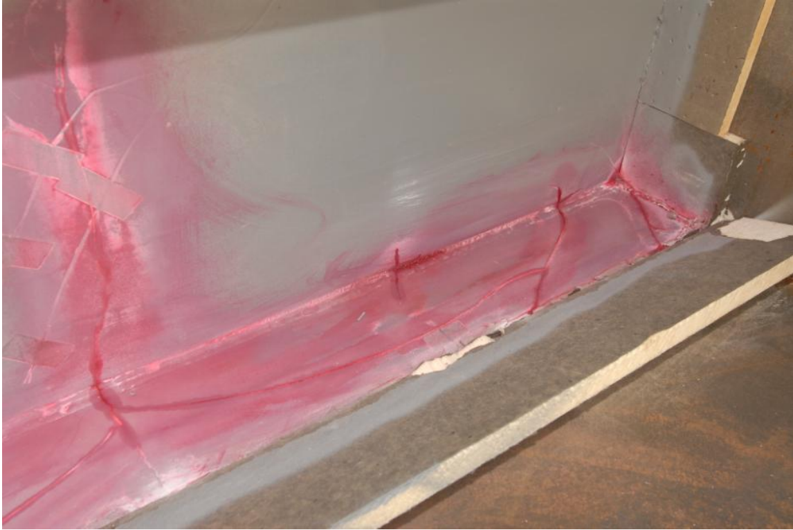
Figure 55. Outside cracking with turning for Test 16
