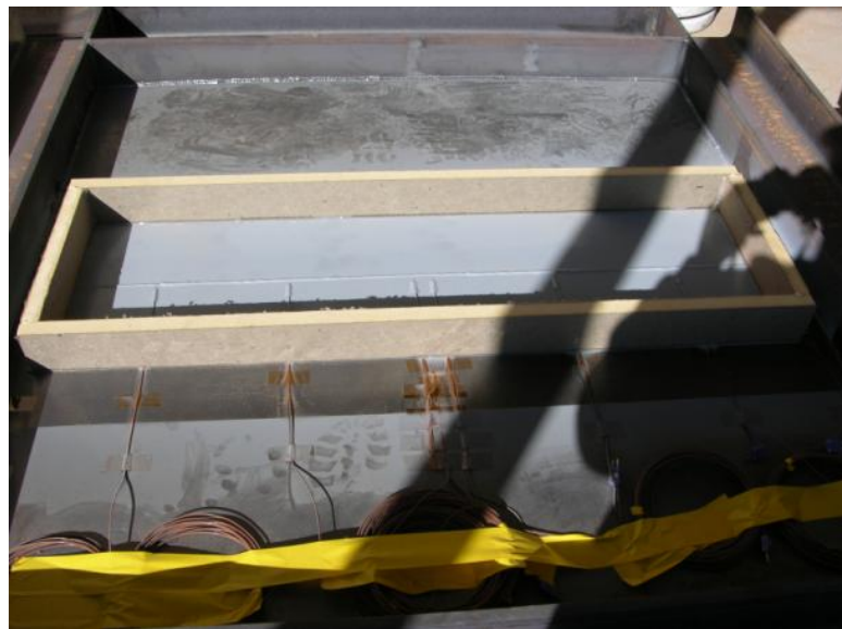
Figure 10. Welded 48 in. x 48 in. x \frac{1}{4} in. Phase II test plate
