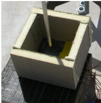
Figure 62. Plate setup used in heat transfer tests
