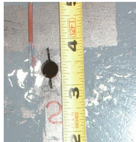
Figure 16. Notched holes for Tests 5 and 6, center hole (hole 2) shown.
