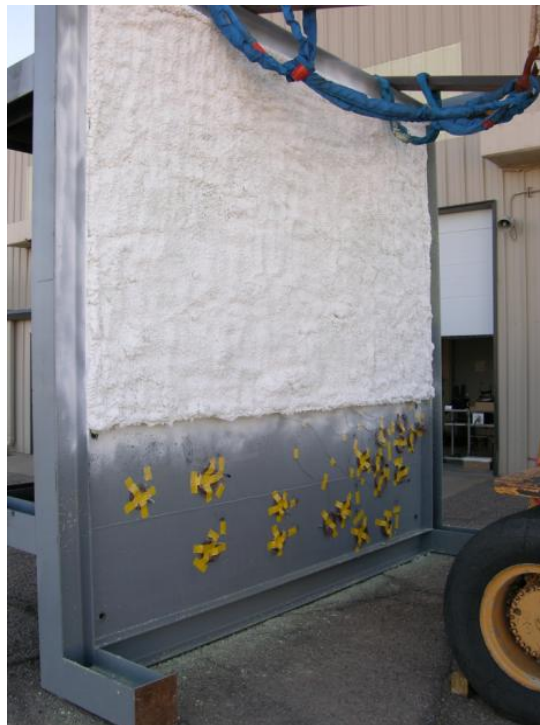
Figure 57. Polyurethane foam applied to the bottom of the large structure
