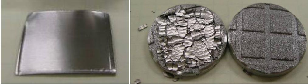
**Figure 6: HCRH sample before (left) and after hydriding at 250 °C.**
