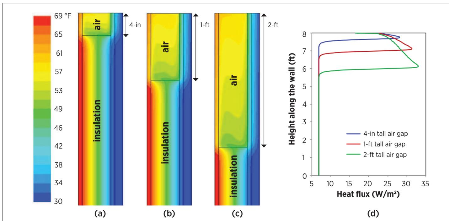
**Figure 1.** (a-c): Temperature distribution in the upper section of a partially insulated wall cavity. (a) 4-in. tall air gap, (b) 1-ft tall air gap, and (c) 2-ft tall air gap. (d): Heat flux along the inner surface of the wall exchanging heat with the room air. These results are for 70°F indoor temperature and 30°F ambient temperature. *Figures by El Hassan Ridouane*
