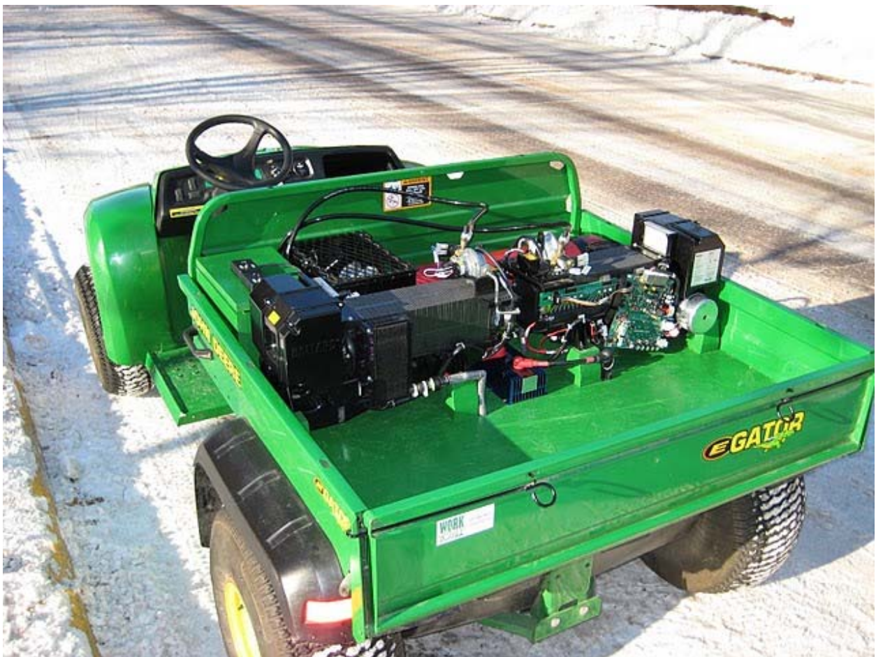
Figure 1. John Deere e-Gator with two fuel cells.
