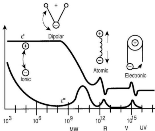
**Figure 1. Dielectric mechanisms as a function of frequency[1].**
