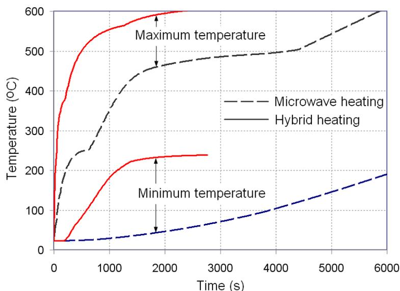
**Figure 9. Time-temperature histories of the maximum temperature in the furnace for microwave and hybrid heating with 2 kW power.**
