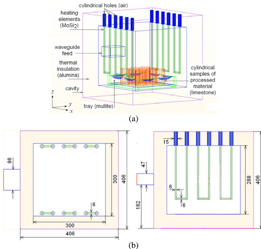
**Figure 6. 3D view of *QW-3D* representation of the MAT<sup>TM</sup> furnace (a) and geometrical characteristics of the furnace's elements (b).**
