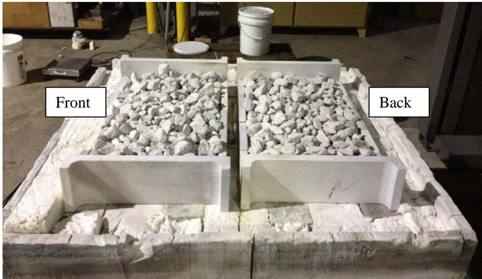
Figure 15. The experimental setup which shows the high alumina kiln furniture positioned into troughs with limestone loaded on the kiln car.
