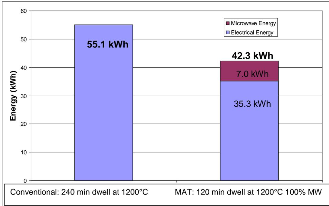
**Figure 13. Energy consumption for 5 kg of limestone calcined to 1200 °C. The conventional weight loss was 41.2%, while the weight loss for the MAT run was slightly higher at 42.3%.**
