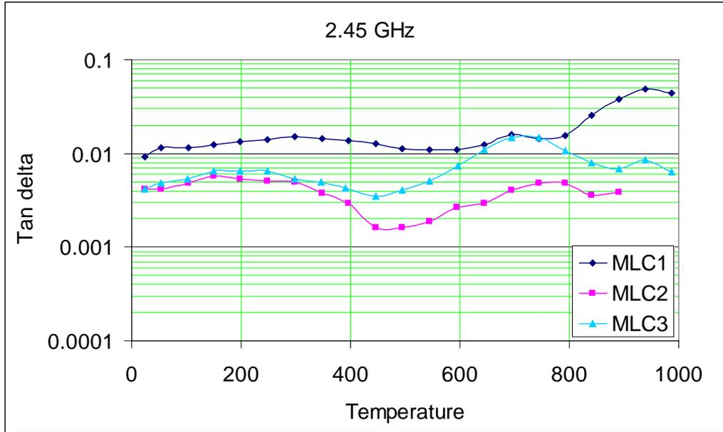
**Figure 2. Tanδ as a function of temperature for 3 grades of limestone. The higher the Tanδ, the better the material should heat by microwave energy.**
