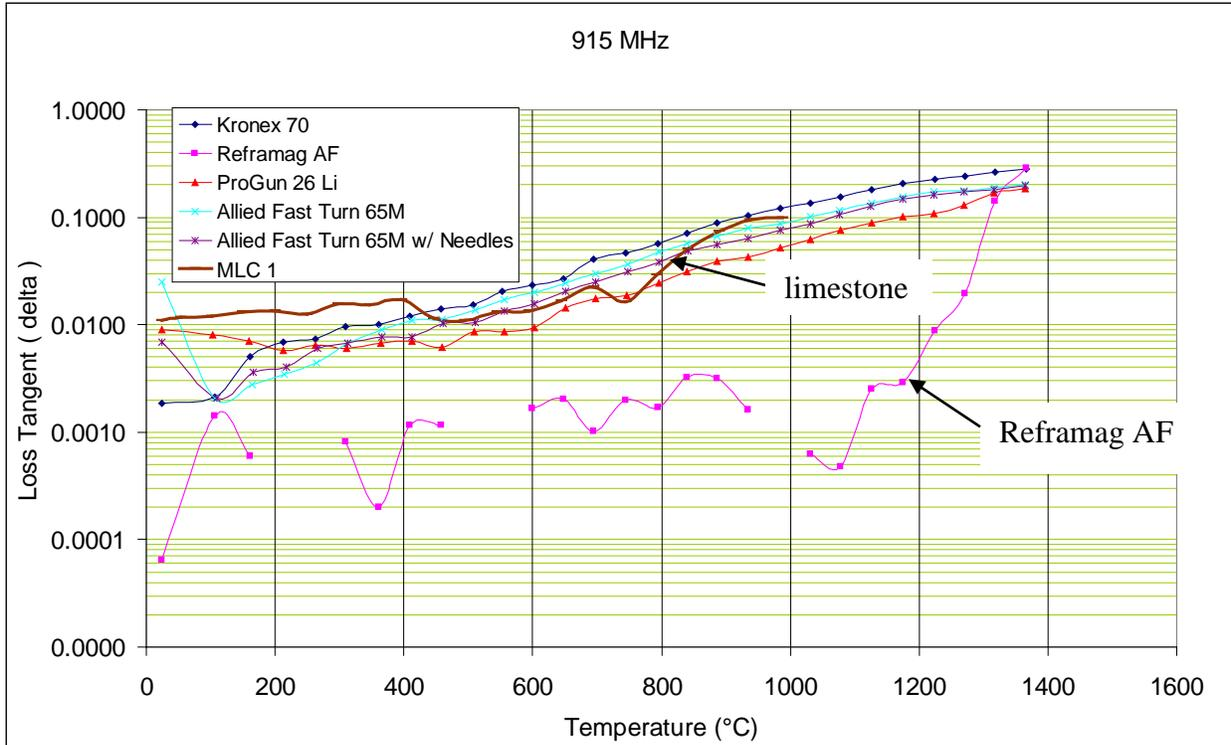
**Figure 3. Graph of the  $Tan\delta$  as a function of temperature for several grades of kiln refractories. Only the reframag AF and ProGun 26 Li had lower  $Tan\delta$  compared to the limestone, making those compatible for microwave processing.**
