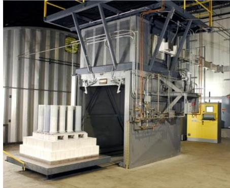
Figure 14. Image of the 27 ft<sup>3</sup> MAT electric 1620 °C kiln at Touchstone.
