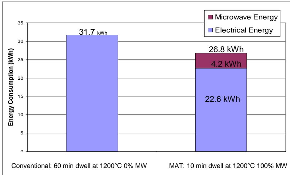
**Figure 12. Energy consumption for 1 kg of limestone calcined to 1200 °C for a weight loss of 43.5%. The MAT run consumed ~18% less energy and 16% less time (0 min dwell time) vs. the conventional with a 60 min dwell time.**
