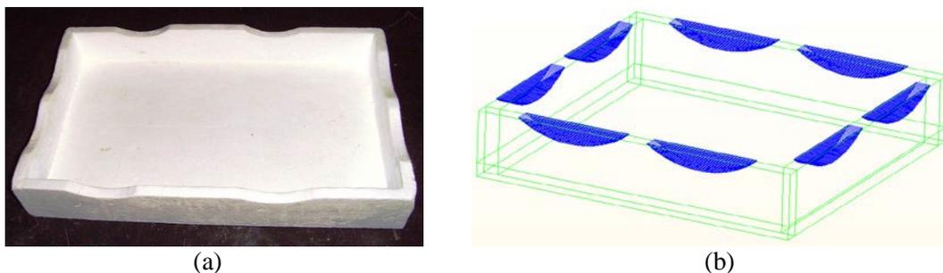
**Figure 5. Mullite tray for the limestone samples – general view (a) and representation of the model (b).**
