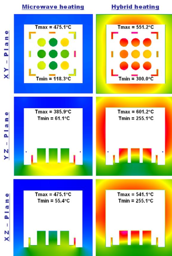
**Figure 10. Temperature distributions in the central coordinate planes after 40 min of heating.**
