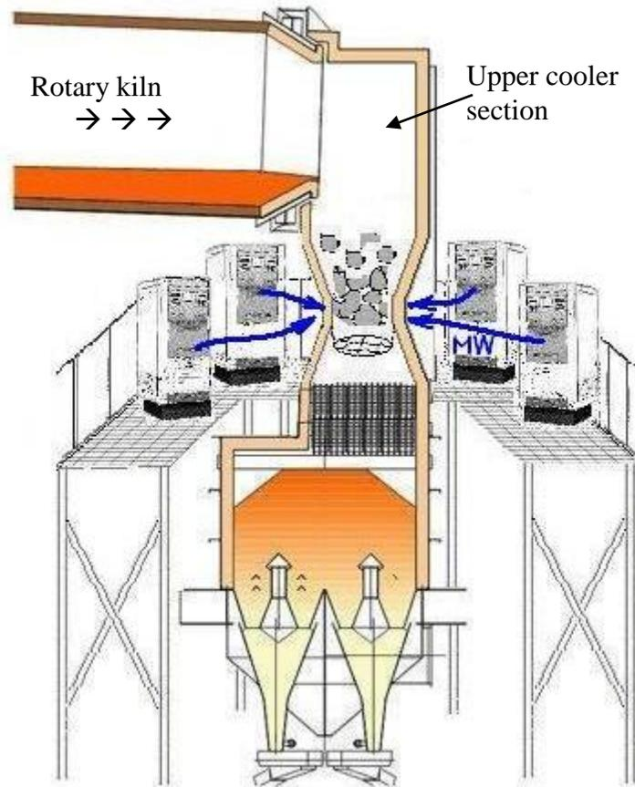
**Figure 16. Sketch of the post-heat section of a rotary kiln with microwave energy applied by four microwave generators and a slimmer section with a diameter of 6 ft and a length of 4 ft.**
