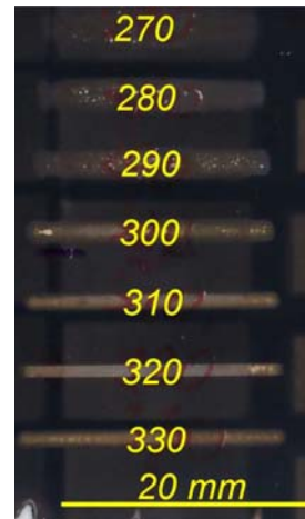
Figure 7. Relative laser power density (as displayed on thermally-sensitive paper) as a function of laser stand-off distance (mm). Focal distance of 320 mm yields the smallest laser “foot print”, which corresponds to the higher power density for surface heating.
