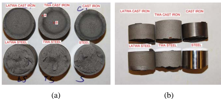
Figure 21. Cut sections from the failed fatigue tested bars, (a) fracture surface, (b) surface close to the fracture
