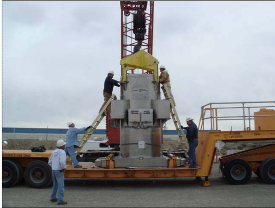
Figure 2-7. 55-ton scrap cask used for transporting waste to a disposal facility.
