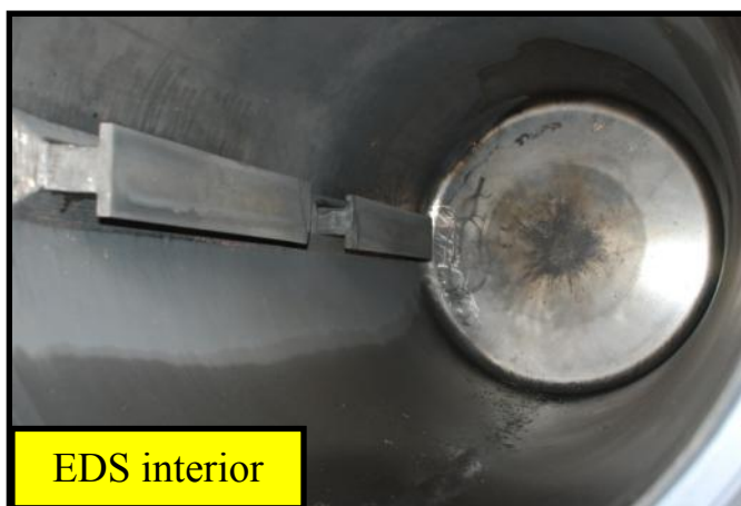
Figure 11: Representative condition of EDS vessel interior surfaces following detonation and de-pressurization. Blast marks (non-damaging) are evident on flat door and end (aft) surfaces.
