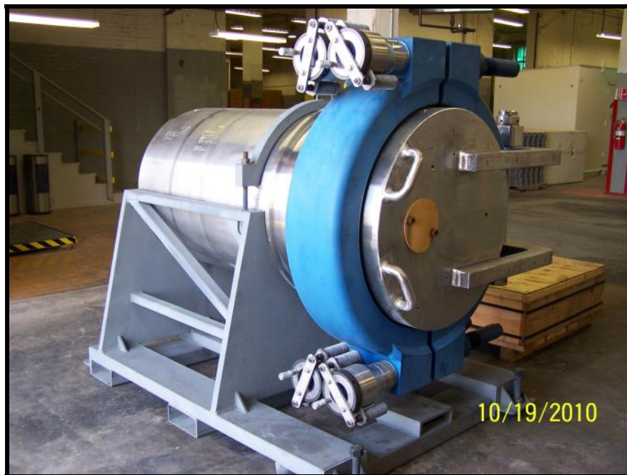
Figure 1: This image shows the EDS vessel mounted in the shipping fixture.
