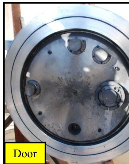
Figure 11: Representative condition of EDS vessel interior surfaces following detonation and de-pressurization. Blast marks (non-damaging) are evident on flat door and end (aft) surfaces.
