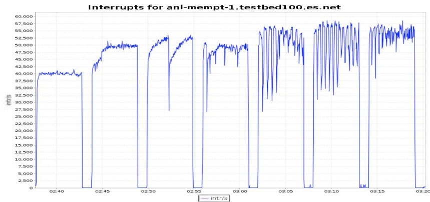
Figure 11: ANI testbed 100Gbps (10x10NICs, three hosts): Interrupts vs the number of concurrent transfers [1, 2, 4, 8, 16, 32 64 concurrent jobs - 5min intervals], TCP buffer size is 50M
