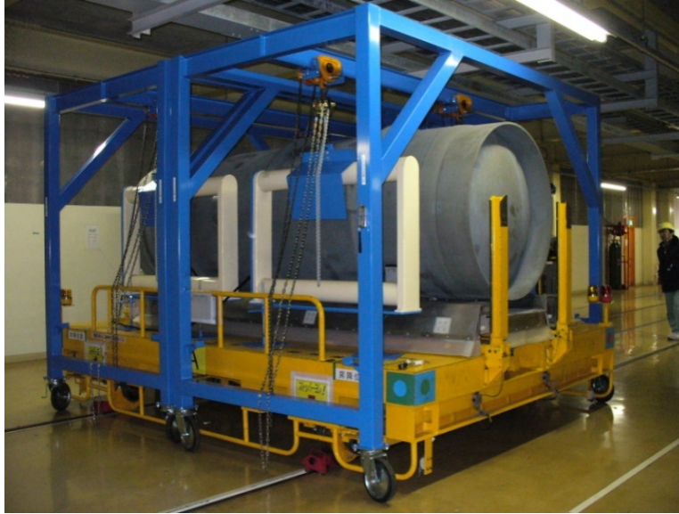
Fig. 2. The PNEM measurement concept grew out of the success of the Uranium Cylinder Assay System (UCAS). The UCAS is shown here with a 48Y cylinder at Rokkasho Enrichment Plant (REP) in Japan.
