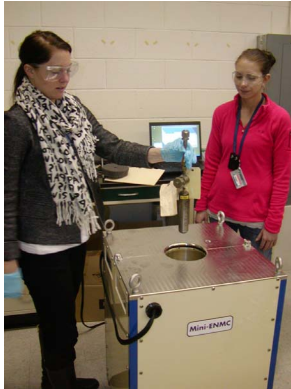
Fig. 10. Extension of the PNEM measurement technique to small \text{UF}_6 cylinders using the Mini-Epithermal Neutron Multiplicity Counter (Mini-ENMC) at LANL's Sigma Facility.
