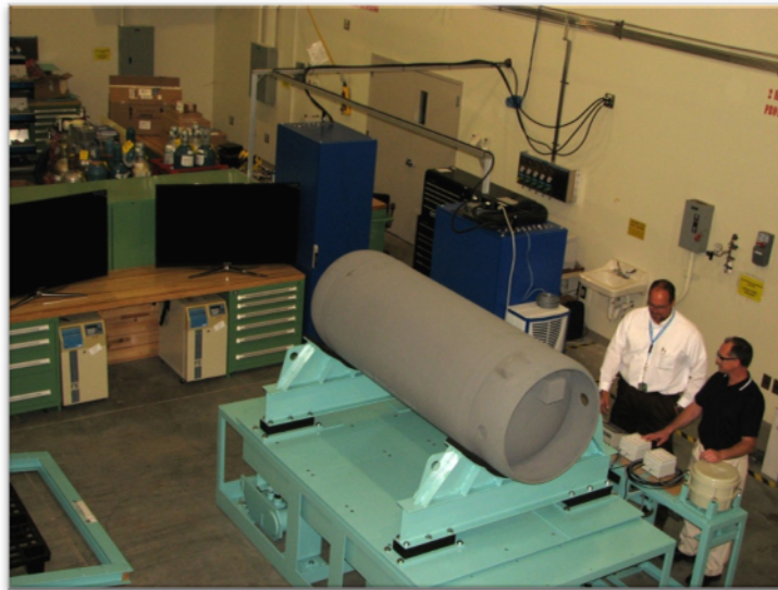
Fig. 8. This photograph shows SRNL's \text{UF}_6 cylinder measurement test bed, which includes an accountancy scale inside a tamper-indicating enclosure (photograph provided by SRNL).
