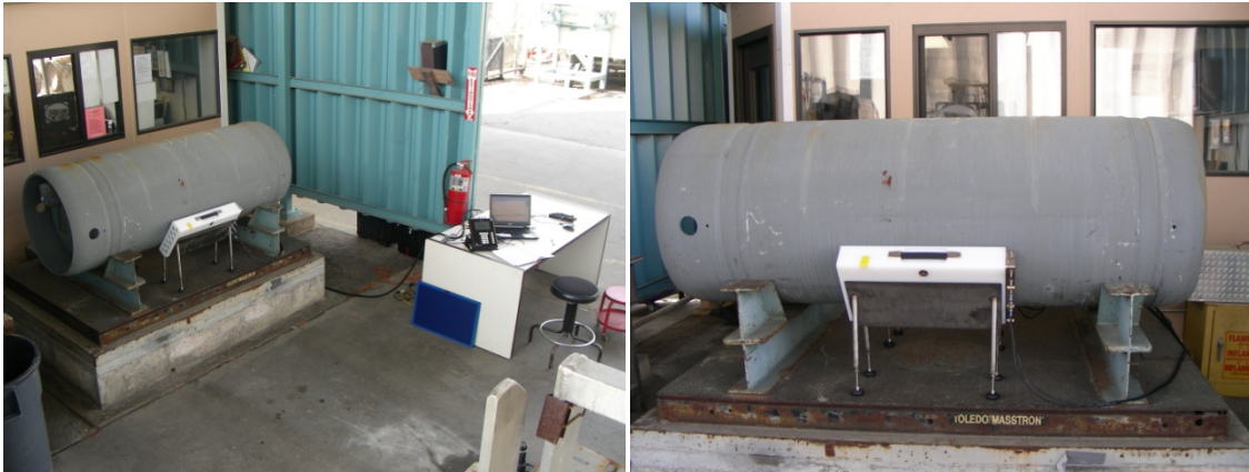
Fig. 9. The measurement configuration for the March 2012 PNEM field trial at WFFP that combined the neutron detection system with the existing scale at WFFP.
