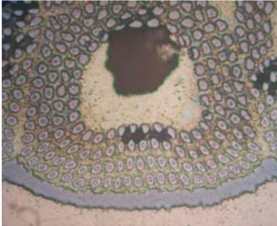
**Figure 7a:** Micrograph of an unstrained Luvata ITER wire reacted at 650 °C for 100 hours (Short HT). There is a significant number of unreacted cores inside the filaments. These unreacted cores are believed to act as crack initiators (M. Jewell et al., Florida State University). Image courtesy of T. Pyon, Luvata Waterbury Inc.
