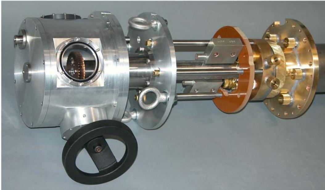
**Figure 1:** Photograph of the upper part of the new high-current apparatus constructed at NIST to measure the critical-current dependence on strain, temperature and magnetic field. The worm-wheel that torques the spring can be seen through one of the windows.
