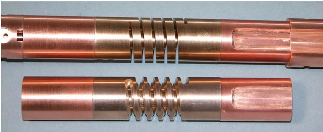
**Figure 2:** Photograph of the two CuBe springs used in the new high-current apparatus: rectangular-section (top) and T-section (bottom) geometries.
