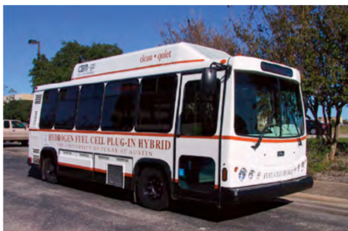
Hydrogen fuel cell plug-in hybrid electric transit bus. Manufactured by Ebus. Located at the University of Texas Pickle Research Center in Austin, Texas. 2008.
