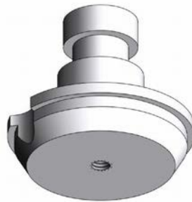
Figure 4.2: Up to 16 of these sample holder heads made of aluminum can be placed in a tray for sequential sample measurements. The alignment notch shown left ensures repeatability of the sample position. A sample can be attached using the standardized 10-32 screw hole shown on the bottom. Figure originally published in my paper [48].
