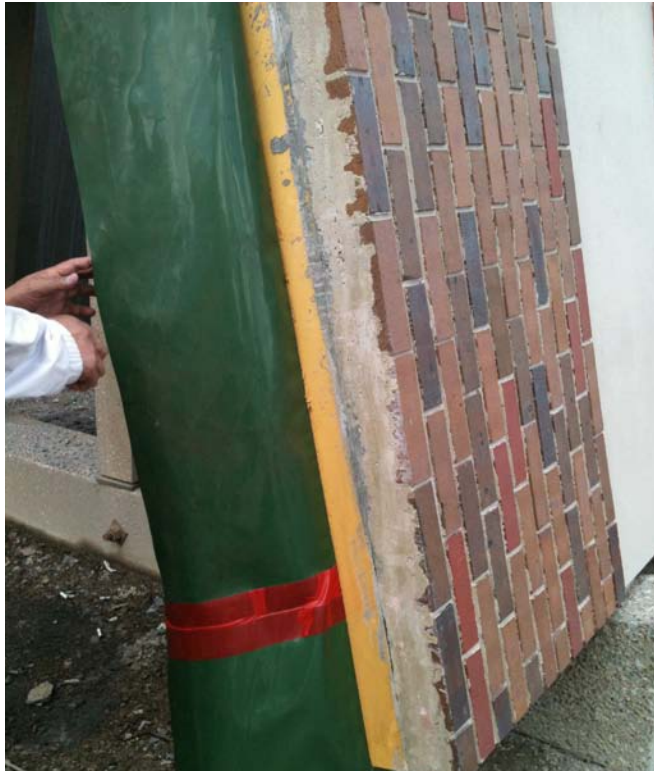
Figure 7 Same wall section but picture taken to show the finished front surface, then the polyiso and moisture barrier
