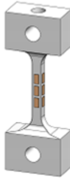
Figure 7: Alignment specimen with strain gages affixed. When in alignment, all the strain gages should produce the same output.
