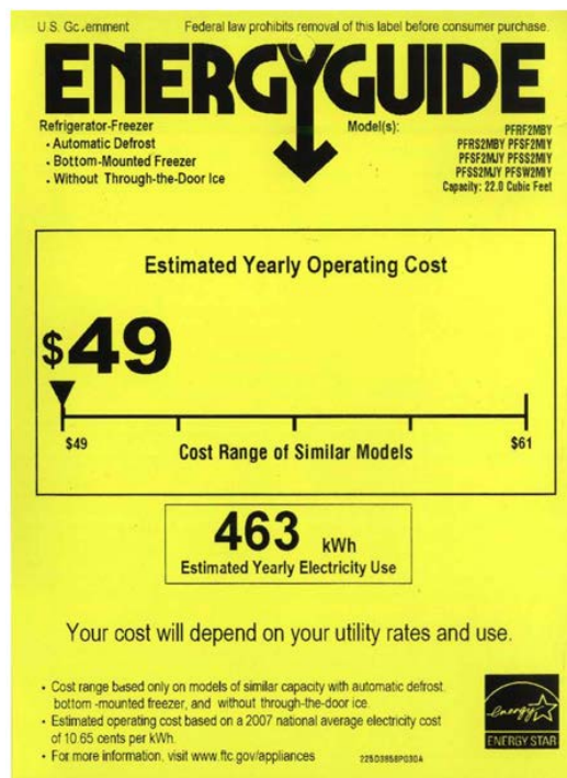
Figure 15. Energy Guide Label for new bottom freezer ENERGY STAR GE refrigerator
