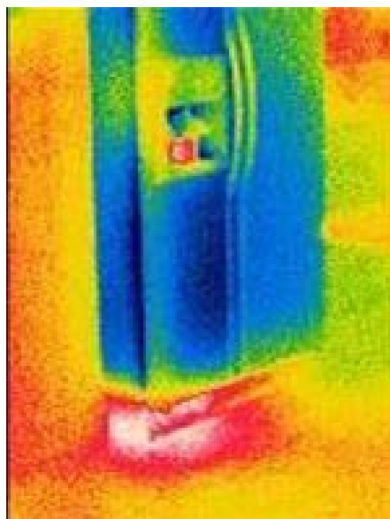
Figure 12. Infrared image of 25-ft 3 refrigerator showing heat rejection at the base of the unit, but also warm temperatures near through the wall ice and water access. The unit was using 4.4 kWh/day prior to replacement in January 2011.
