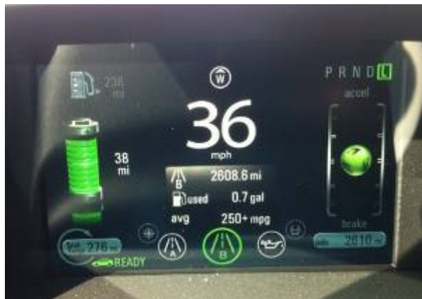
Figure 85. On board display on February 2, 2012 showing 2,609 miles driven with only 0.7 gallons of fuel consumed. At this point, 776 kWh had been used at home to charge the car which had been operated in all electric mode, with gasoline only used for monthly maintenance starts.
