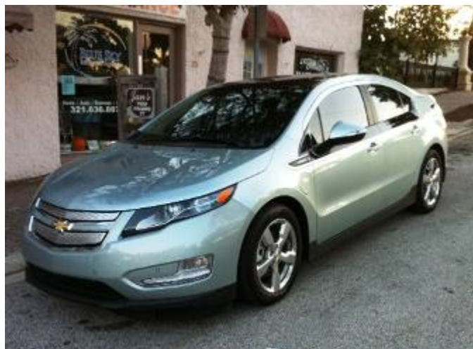
Figure 80. 2012 Chevrolet Volt with an estimated driving range of 35–45 miles on the 10.4 kWh battery
