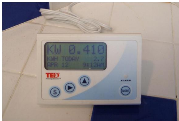
Figure 57. The Energy Detective real-time energy feedback device
