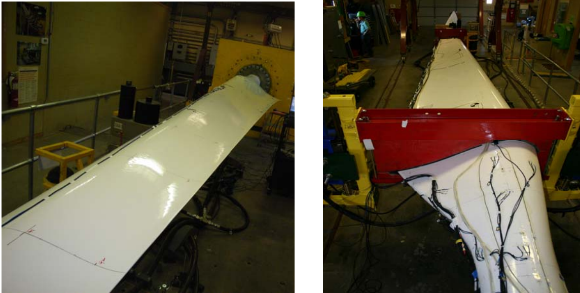
Figure 7. CX-100 blade tested without added mass (left) and with added mass (right).
