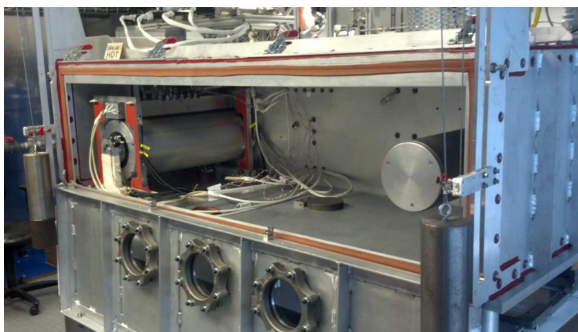
Figure 14 The chamber with the door lowered, showing the drum system at the far end.. The cylinder at the near end of the chamber is part of a system to allow deposition on larger samples.
