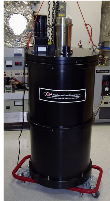
Figure 1. 2 MW CW waterload for Gaussian mode gyrotrons
