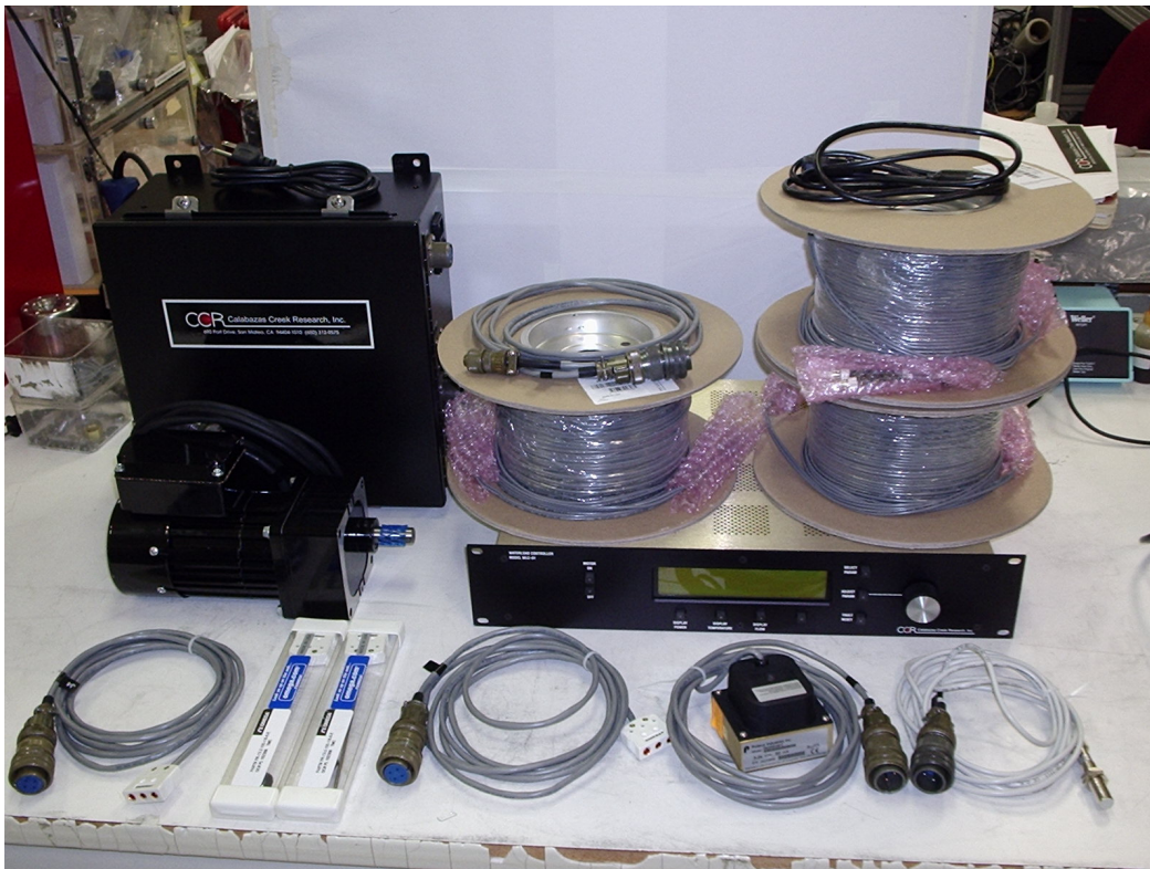
Figure 7. Photograph of waterload electronics, including rack mounted controller, RTDs, flow sensor, fiber optic cables, launcher motor, and remote sensor controller.
