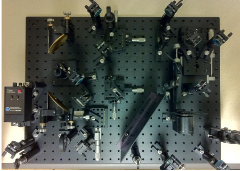
Fig. 7. Photo of a THz TDS system without transmission module.
