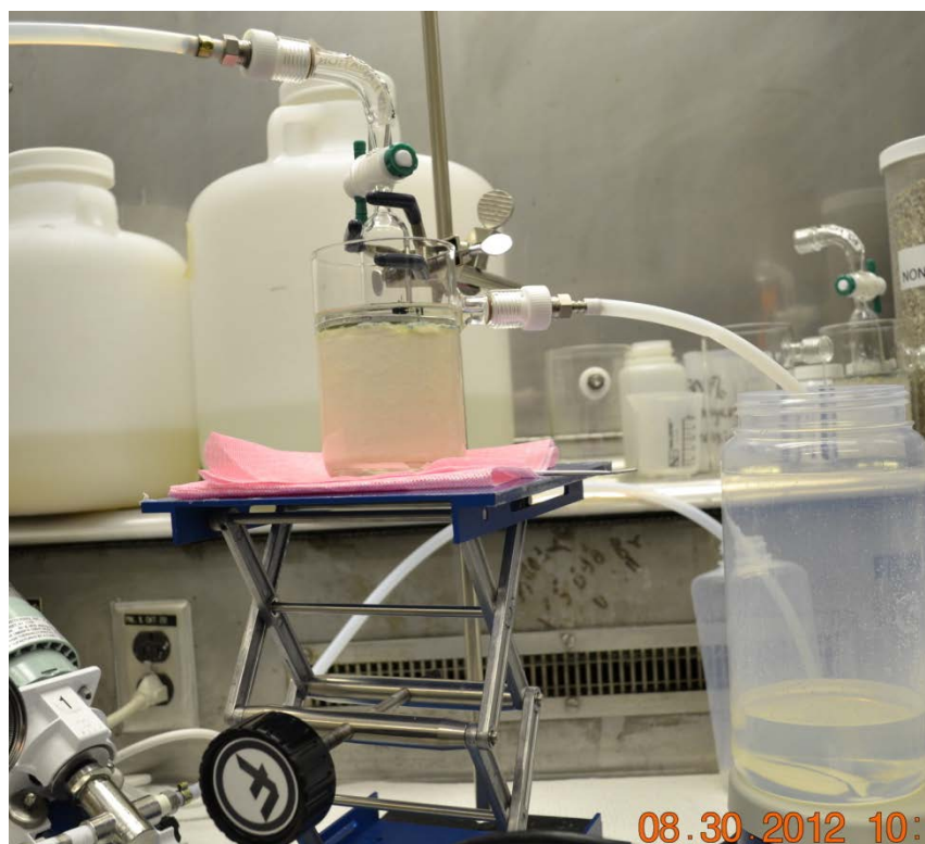
Figure 2-2. A picture of the coalescer in vertical configuration.
