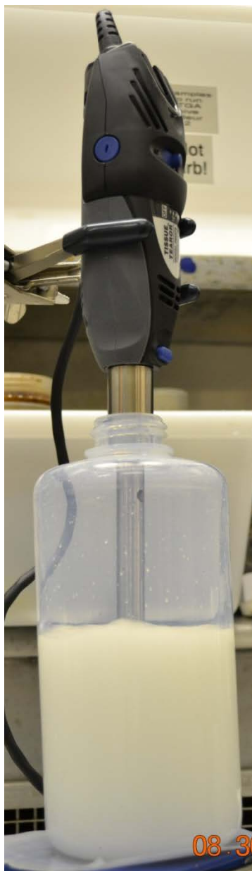
Figure 2-1. Physical appearance of the emulsion obtained using the homogenizer on salt solution containing CSSX solvent.
