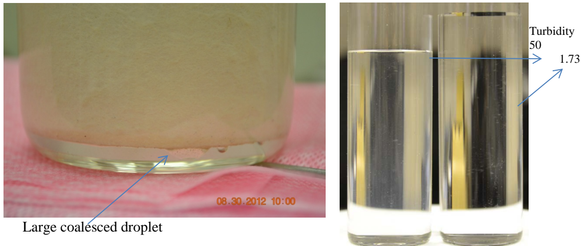
Figure 3-19. Picture of coalesced solvent forming at the bottom of the coalescer. Also shown is the typical turbidity observed 5 minutes and 20 minutes after sending the solution through the coalescer.
