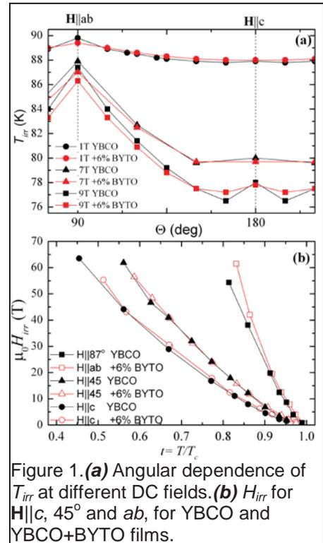
Figure 1. (a) Angular dependence of  $T_{irr}$  at different DC fields. (b)  $H_{irr}$  for  $\mathbf{H}\parallel c$ , 45° and  $ab$ , for YBCO and YBCO+BYTO films.
