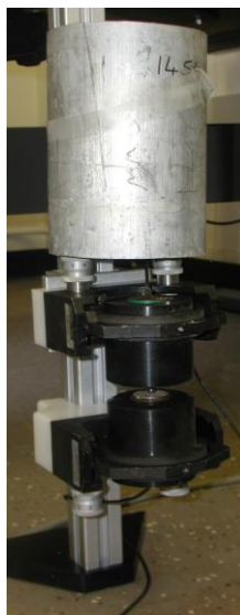
Figure 40. RUS fixture with 14.5 lb weight
