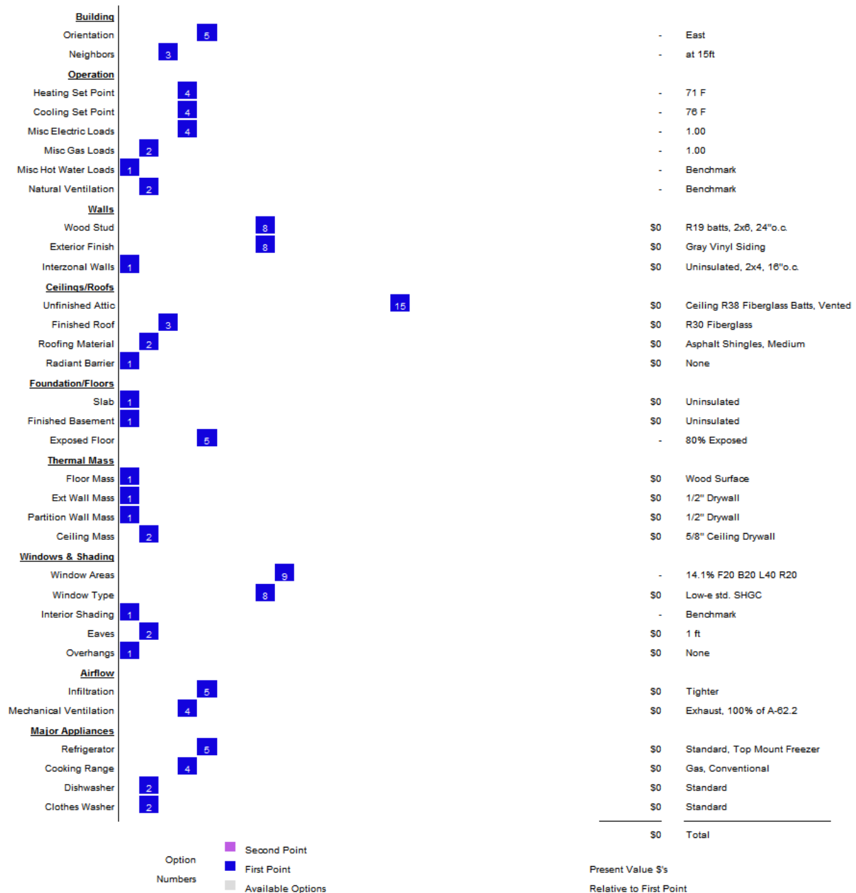
Figure 19. Full basement BEOpt model house specification
