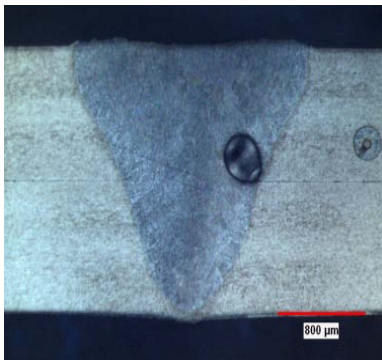
Figure 9: Weld cross-section from practice coupon corresponding to revised EBW parameters of Table 2. Large gas pore is observed originating from lap interface.
