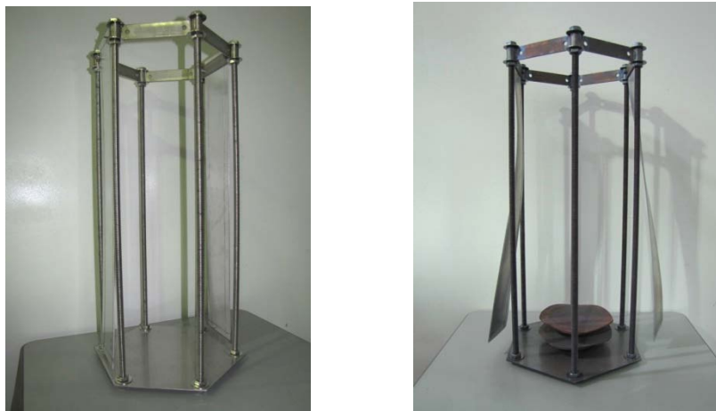
Figure 11: HIP fixture with hanging canless surrogate fuel foil assemblies a) before HIPing and b) after HIPing. Foils are observed to have both bend and twist distortion as a result of HIP operation.
