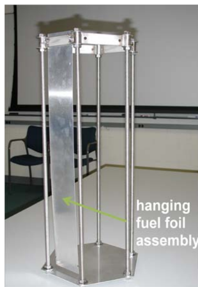
Figure 6: New HIP fixture made specifically for canless HIP processing of 24-inch long foils. Foils are clamped at the top of the fixture and hang freely.
