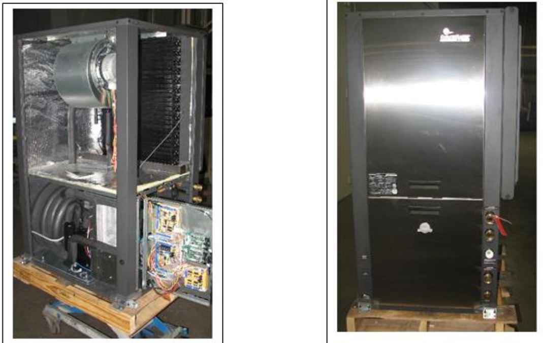
Fig. 4. CM's 1 st generation packaged (field evaluation) prototype GS-IHP unit – l) panels removed with prototype control board pulled out for viewing; r) with all exterior panels in place.
