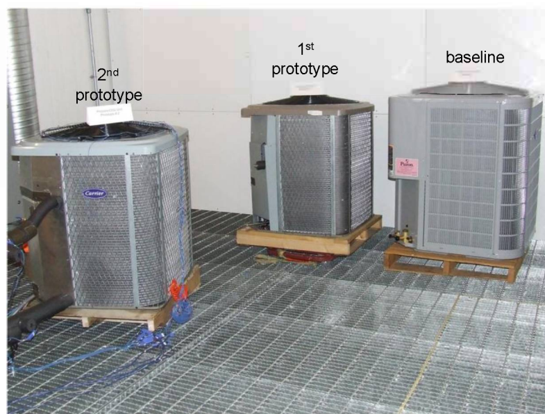
Figure 4.1 Size comparison of the 1 st and the 2 nd prototype outdoor units with the baseline outdoor unit.
