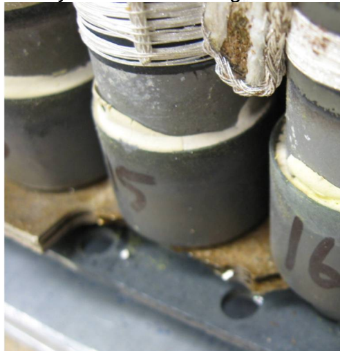
Figure 43 Cemented Joint after 9000 hrs
