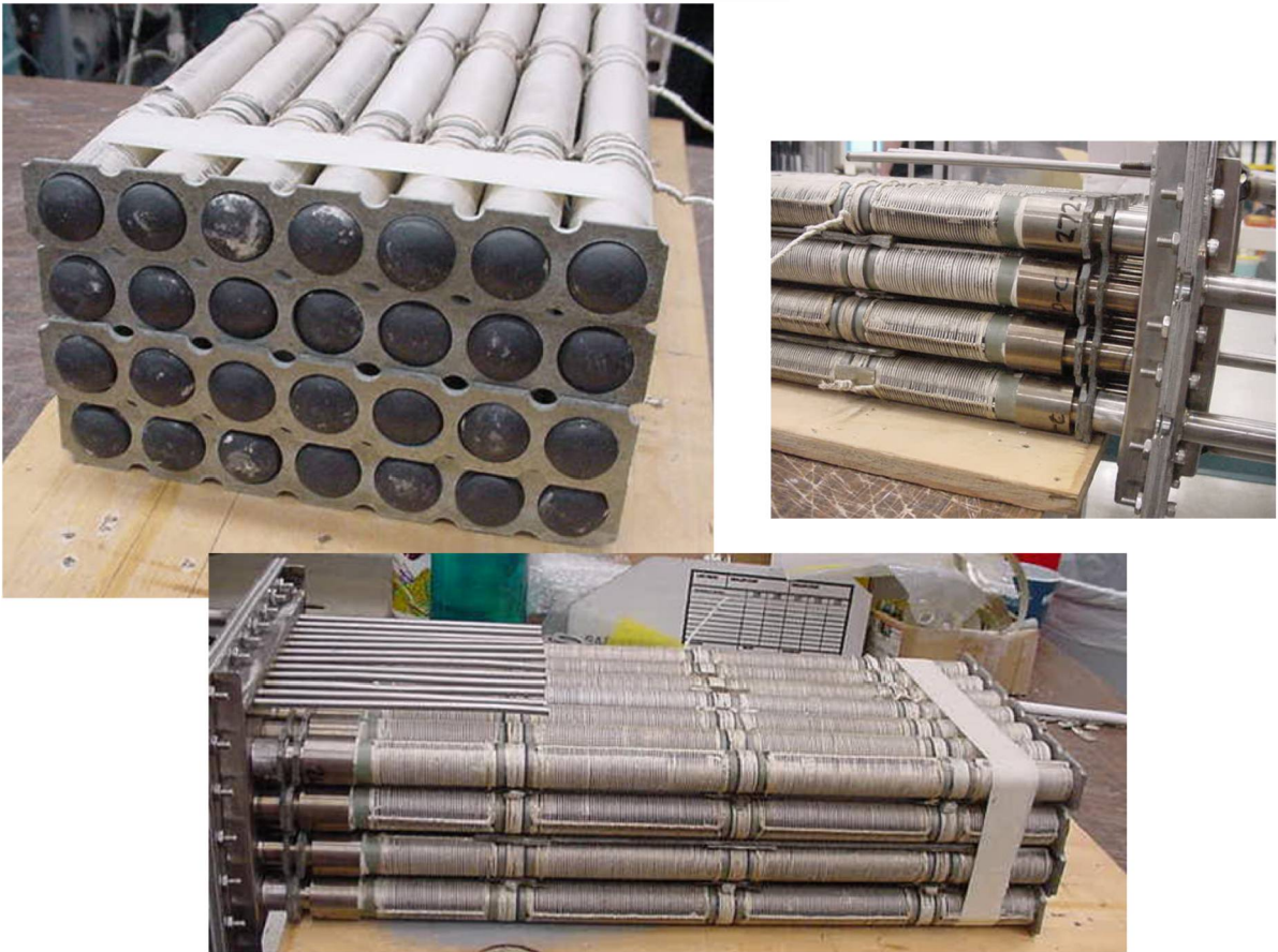
Figure 10 Sintered Bundle with 22 mm Diameter Cells
