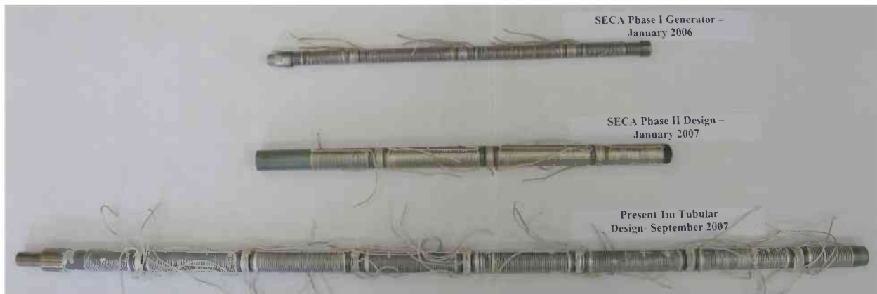
Figure 2 Progression Of Cell Design To Current 125W Cell
