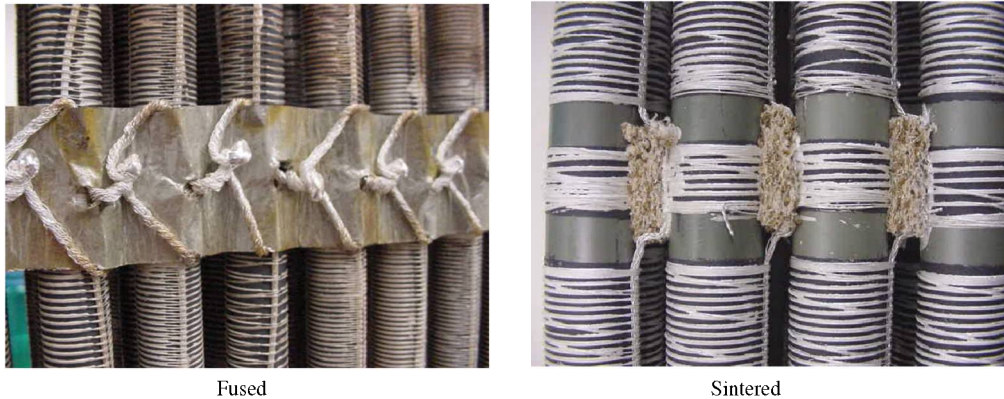
Figure 9 Fused and Sintered Current Collection Methods
