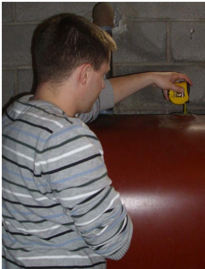
Figure 6. Photo of oil tank level being measured with a tape measure.
